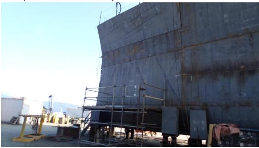
• Sally Ride Pilot House - Inspected pilot house and pilot house void structural welds. ABS in attendance. Found one missing skip weld and one weld with porosity. Both were repaired immediately as pictured below.
