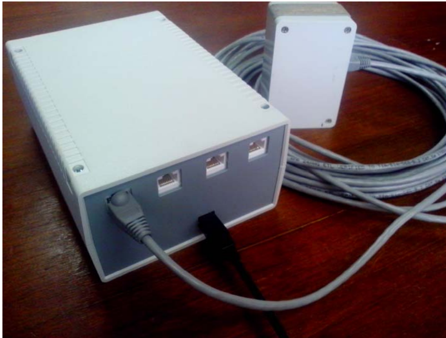
Figure 7: Locator box with UTP connected receiver front-end
