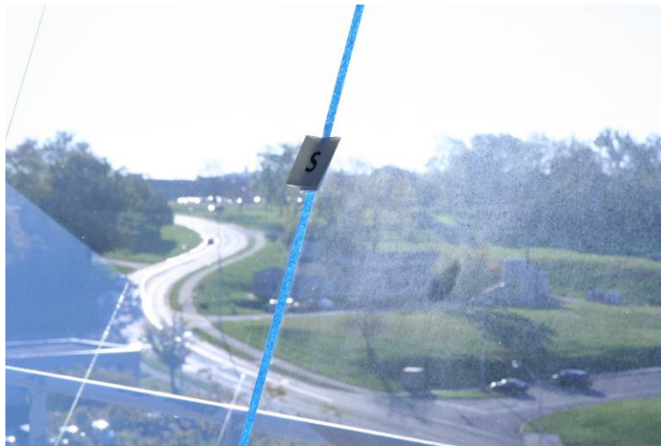
Figure 8. Contrast loss on coated side (right of blue tape) due to light scatter from rising sun.
