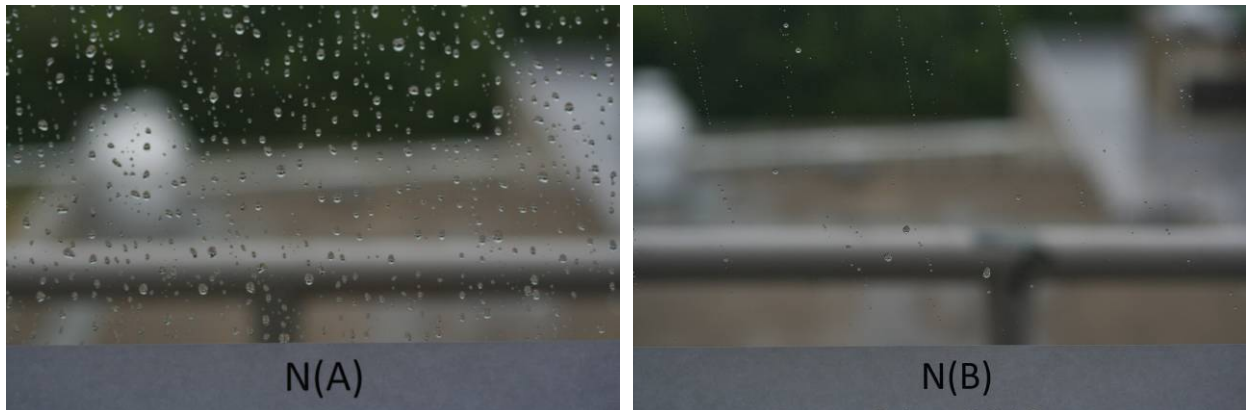
Figure 5. Effect of coating on distribution of water droplets from rain (left is uncoated, right is coated).
