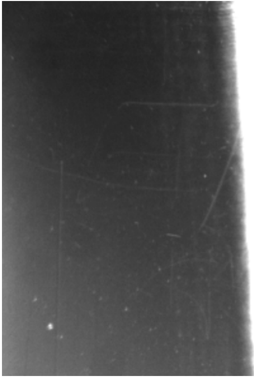
Figure 2: Image of the knife edge used to compute the pre-sampled MTF of the imaging system. The image was acquired using a peak transducer voltage of 0.7 V. Continuous frequency sweeping of 3.25-3.45 MHz at 100 MHz/s was also employed to minimize speckle artifacts due to acoustic wave coherence.
