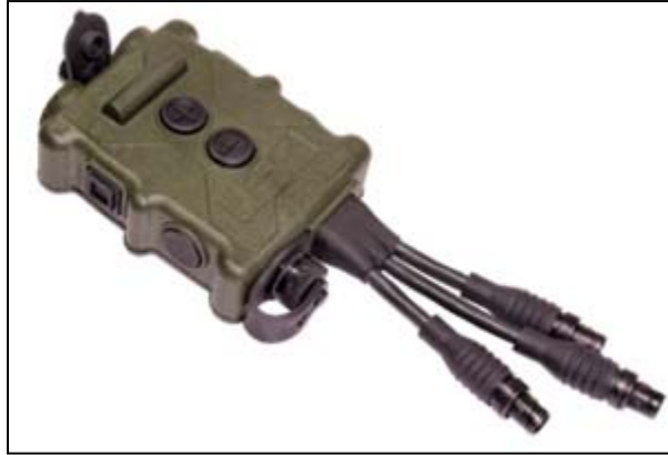
Figure 2. SELEX CTX communications hub.
