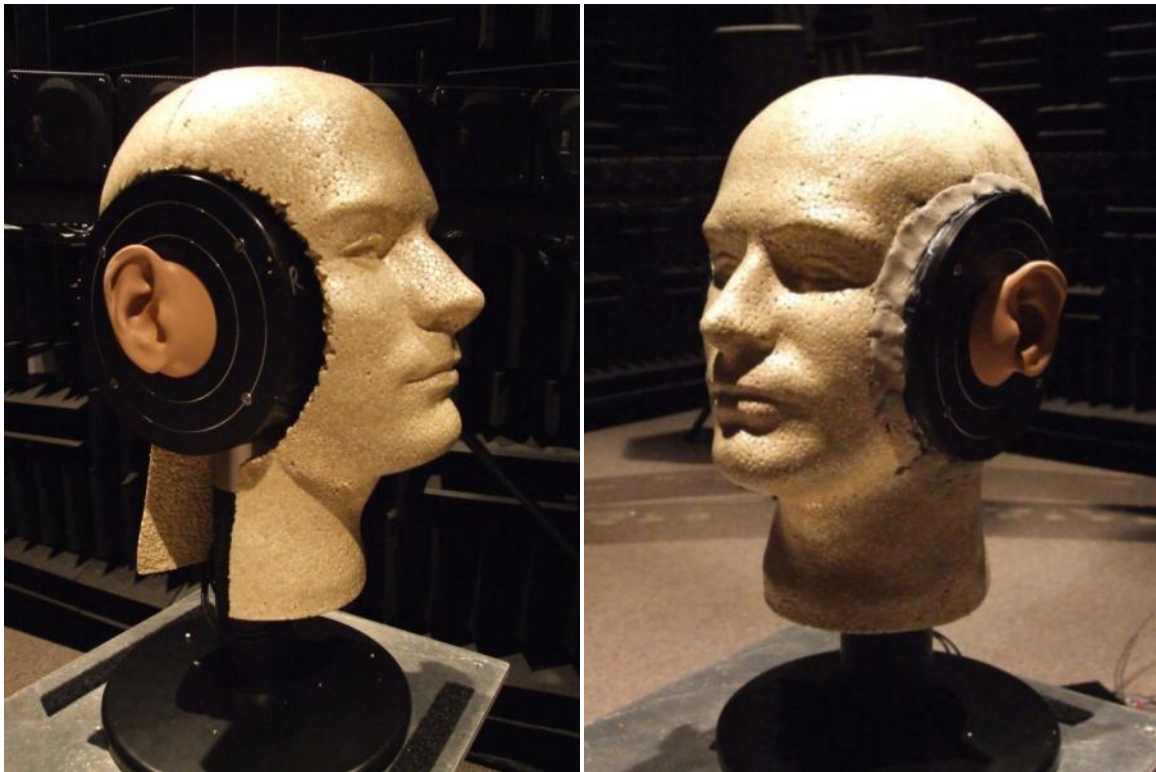
Figure 3. Modifications of the G.R.A.S. 45 Hearing-Protector Test Fixture Type CA used to accommodate helmet testing. Left: the ATF inserted into the manikin head. Right: View with thumb-gum used to seal the manikin to the ATF.
