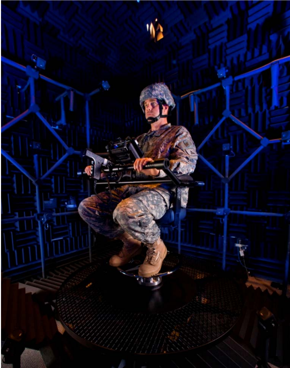
Figure 17. Testing setup used for the localization test in the EAR's Sphere Room (shown with ACH not used in this experiment).
