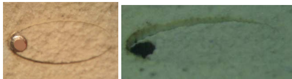
Figure 10: Simple slope shaping of the TBC
