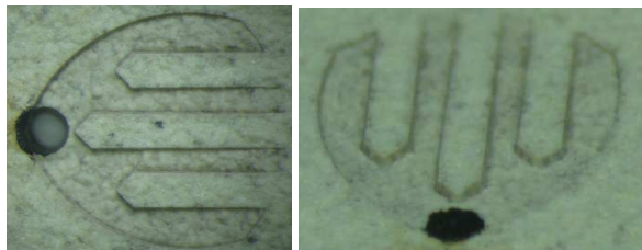
Figure 11: Complex TBC shaping with finger design.
