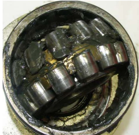
Figure10. Inspection on MIL-PRF-10924H after PNS test
