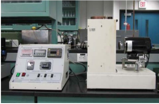
Figure 1. ASTM D3527 Grease Life Test Apparatus
