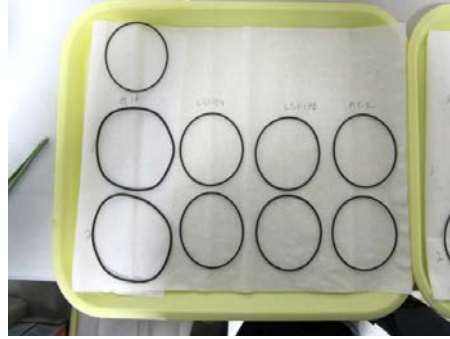
Figure 2. Elastomer compatibility test results with GIA and other candidate greases
