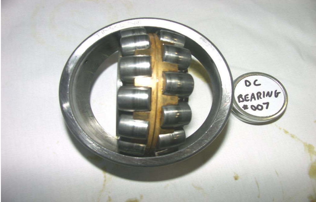
Figure 14. No corrosion or severe wear on bearing roller
