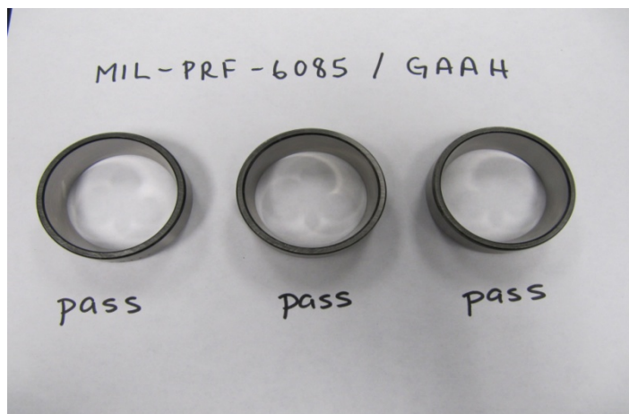
Figure 6. Corrosion/Compatibility Test with MIL-PRF-6085 and GAAH
