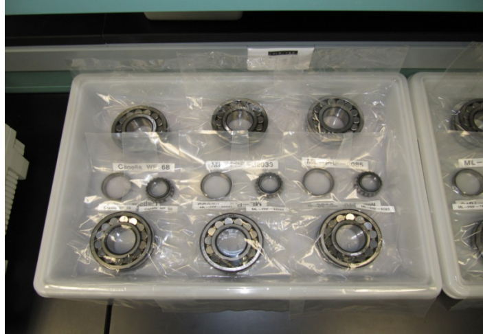
Figure 4. Storage Stability Test of Candidate Preservative Oils in M-G Bearings
