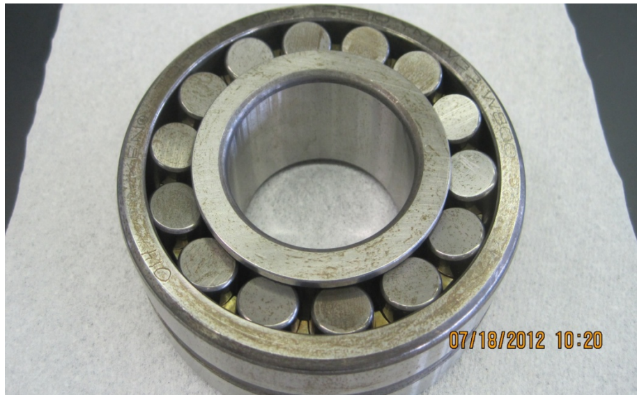
Figure 11. M-G Bearing with stain after cleaning by TBI
