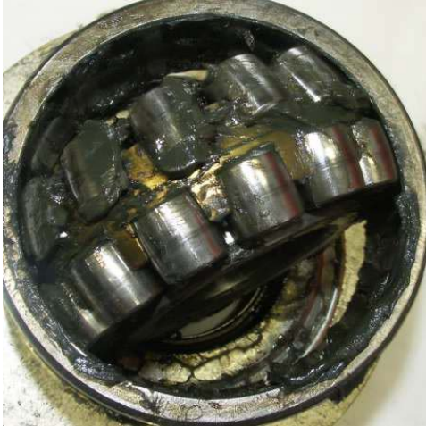
Figure 9. Inspection on 50:50 Mixture Grease after PNS Test
