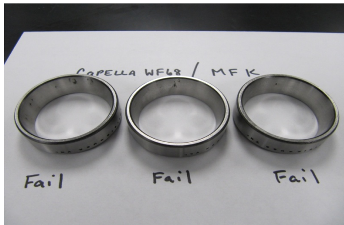
Figure 5. Corrosion/Compatibility Test with Capella WF-68 and MFK
