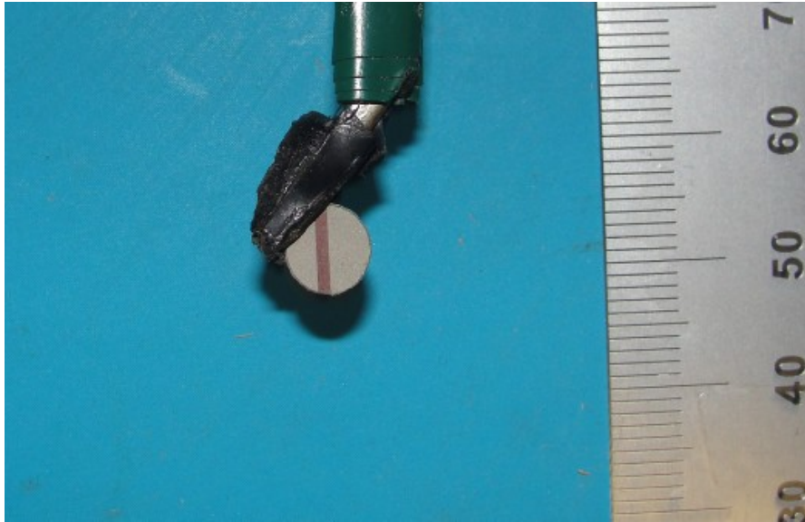
Figure 4-3 Pliers protected with electrical tape are used to hold the PZT sensor.
