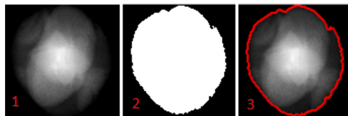
Figure 6.7 The digital image processing used to calculate damage area.
