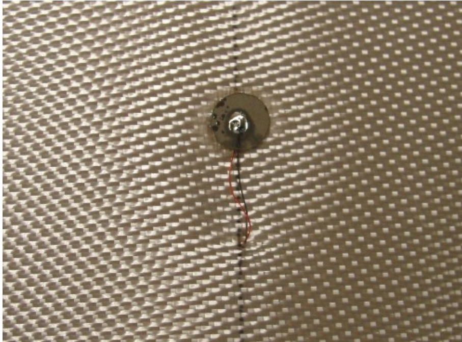
Figure 4-9 Sensor after wire leads are threaded through the glass-fiber layer.
