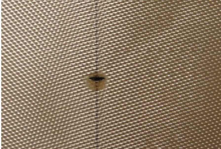
Figure 4-6 Placement of the fast-drying epoxy in the desired position for the PZT. It is important to note that the fiberglass will absorb some of the epoxy in this process.
