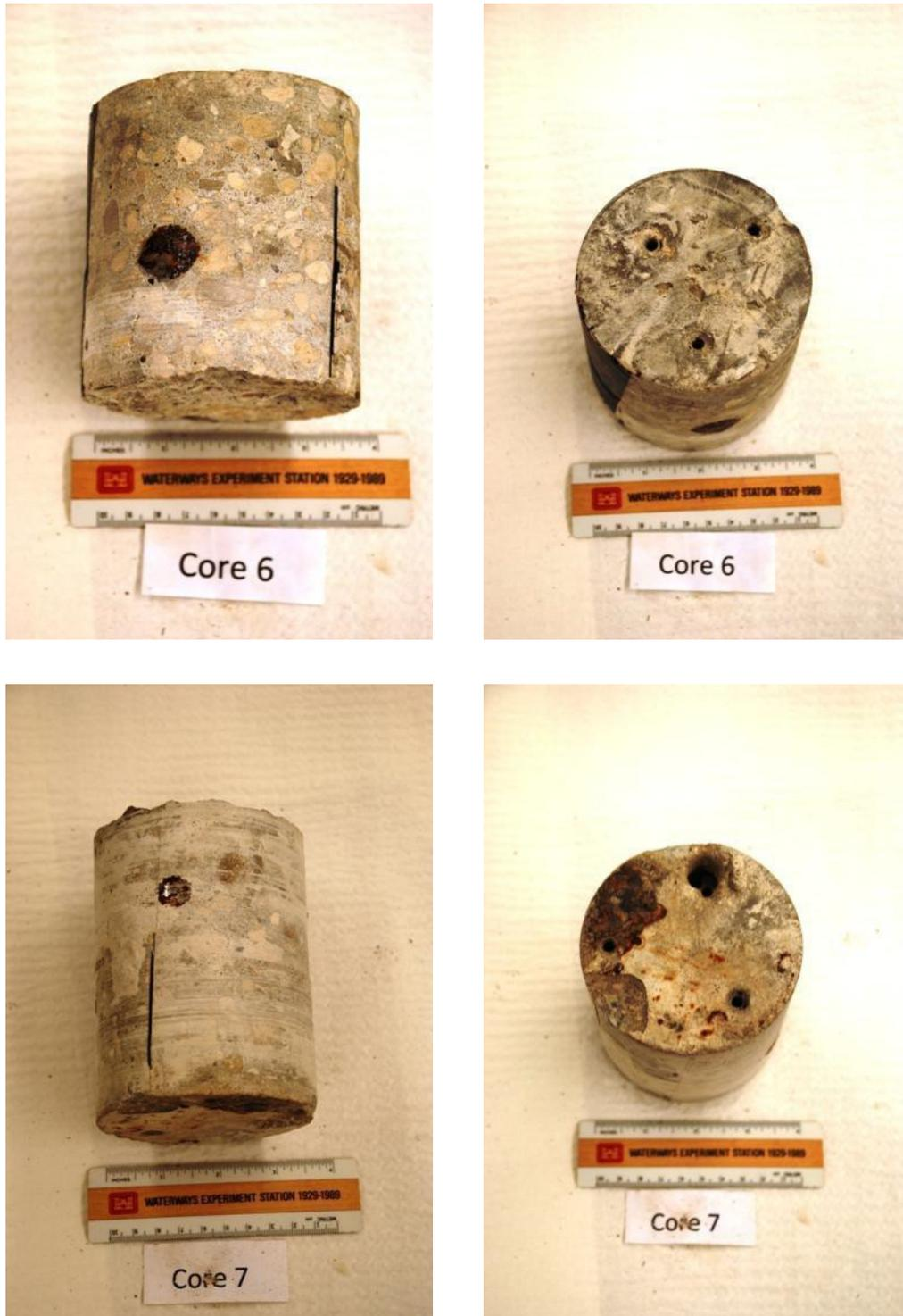
Figure C-3. Photos of as-received core samples #6 and #7.
