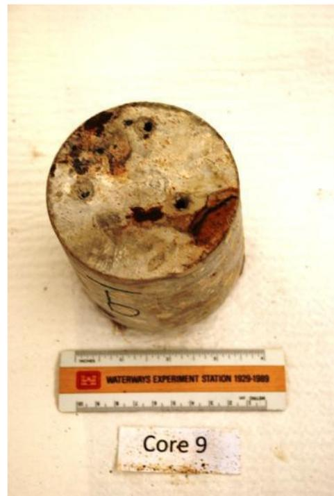
Figure C-4. Photos of as-received core samples #8 and #9.
