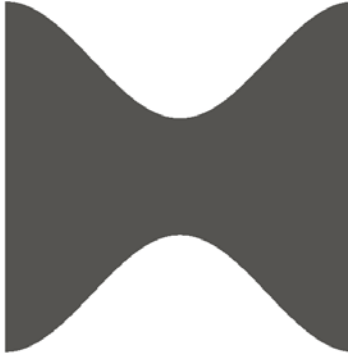
Figure 2: Converging-diverging nozzle used for the Quasi-1D Euler equations.
