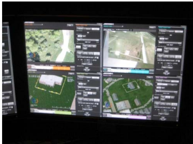
Figure 14-5: Right Control Station Display with Aircraft Video and Sensor Management Area.
