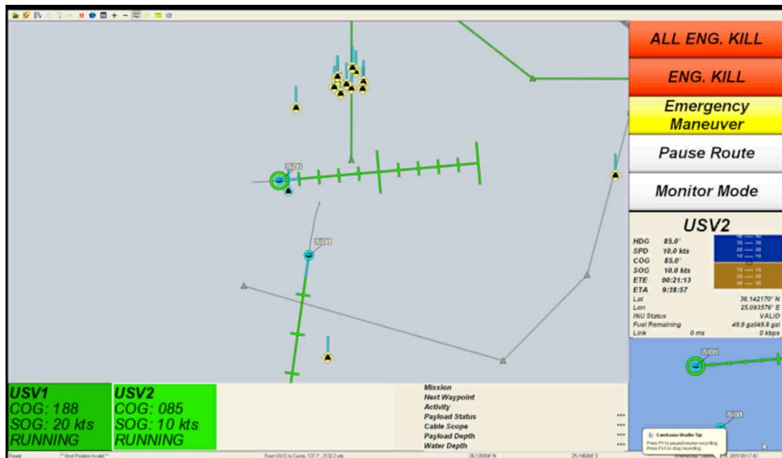
Figure 17-2: Lower Display for Concept 2 Baseline Version of MOCU Multi-USV Chart Information.
