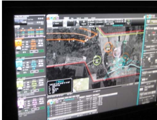
Figure 14-4: Left Control Station Display with System Status Display, Tactical Situation Display, and Vehicle and Payload Controls.
