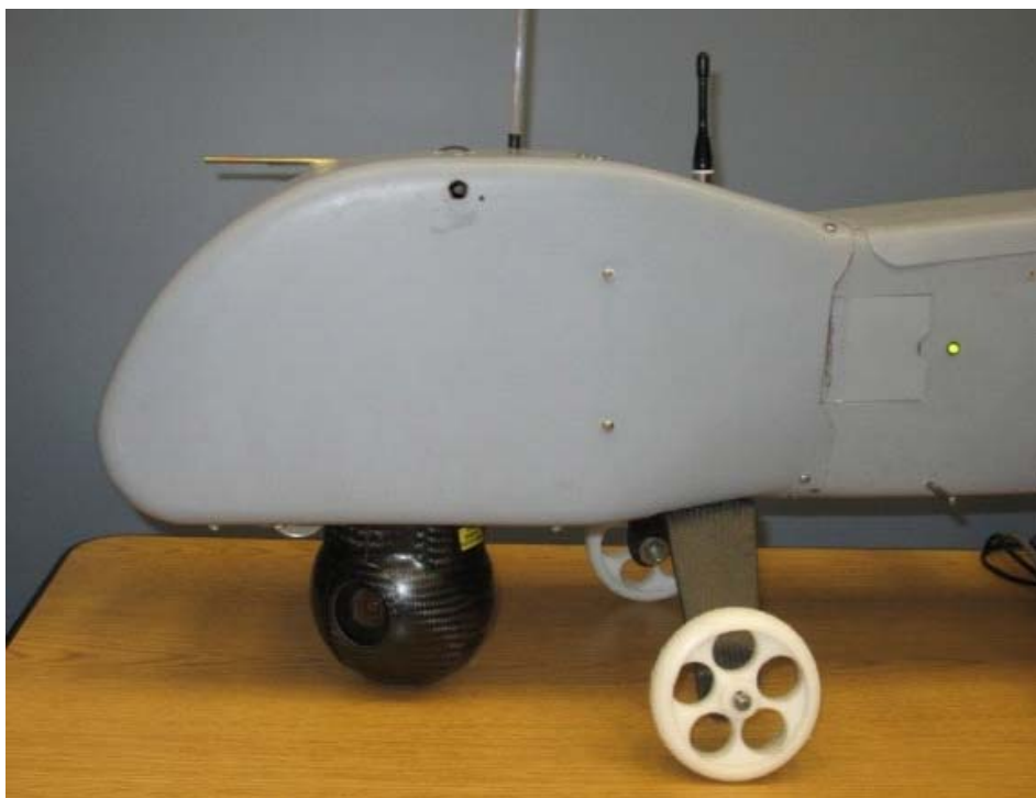
Figure 14-7: Bat 3 with Gimbaled Sensor Deployed.
