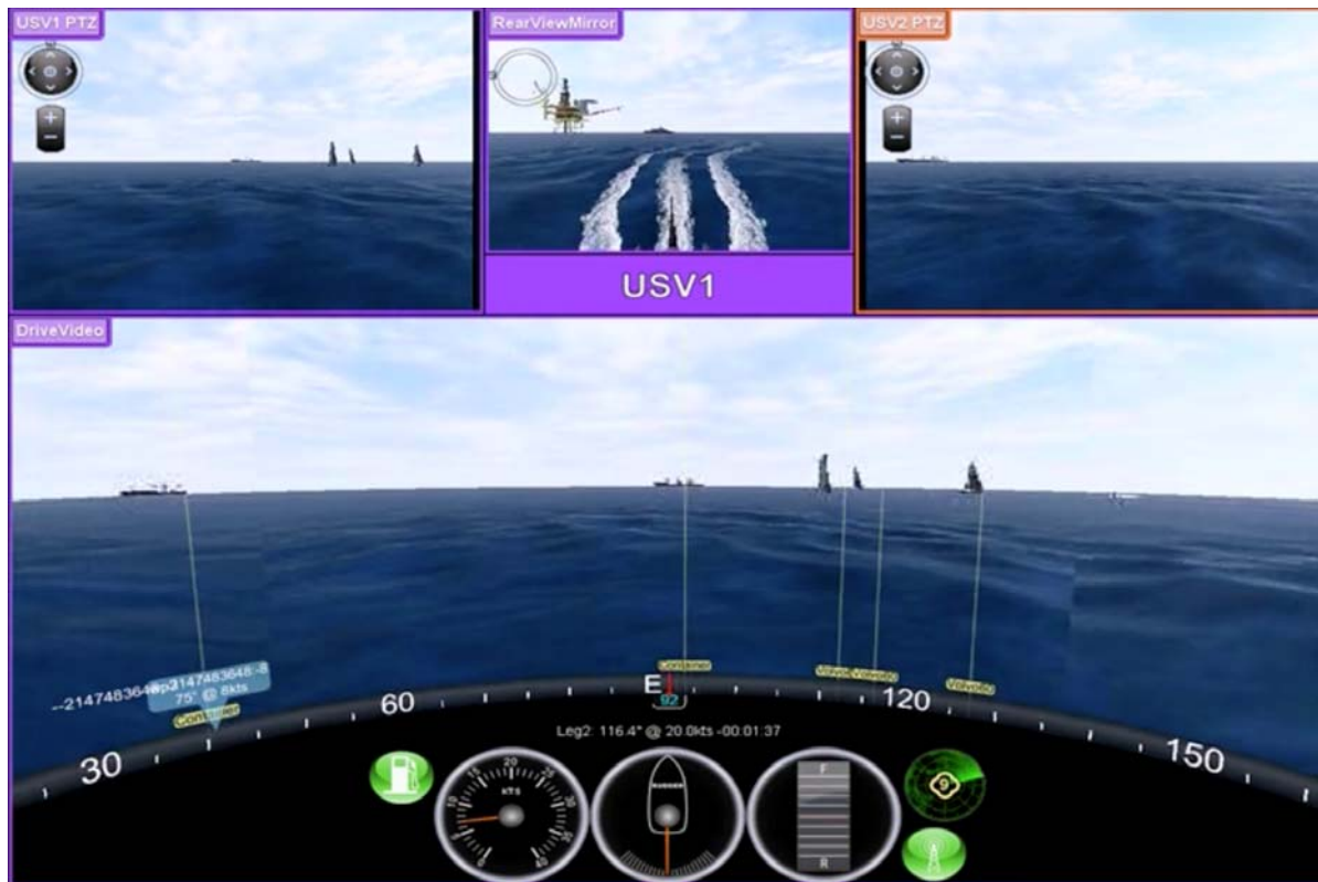
Figure 17-4: Lower Display for Concept 3 Version of MOCU Multi-USV Video Information.
