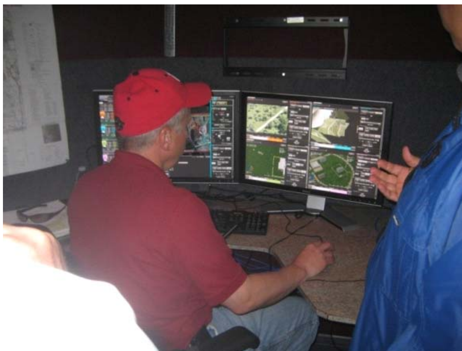
Figure 14-2: Flight Demonstration of Vigilant Spirit Control Station Performing Multi-UAV Operations.
