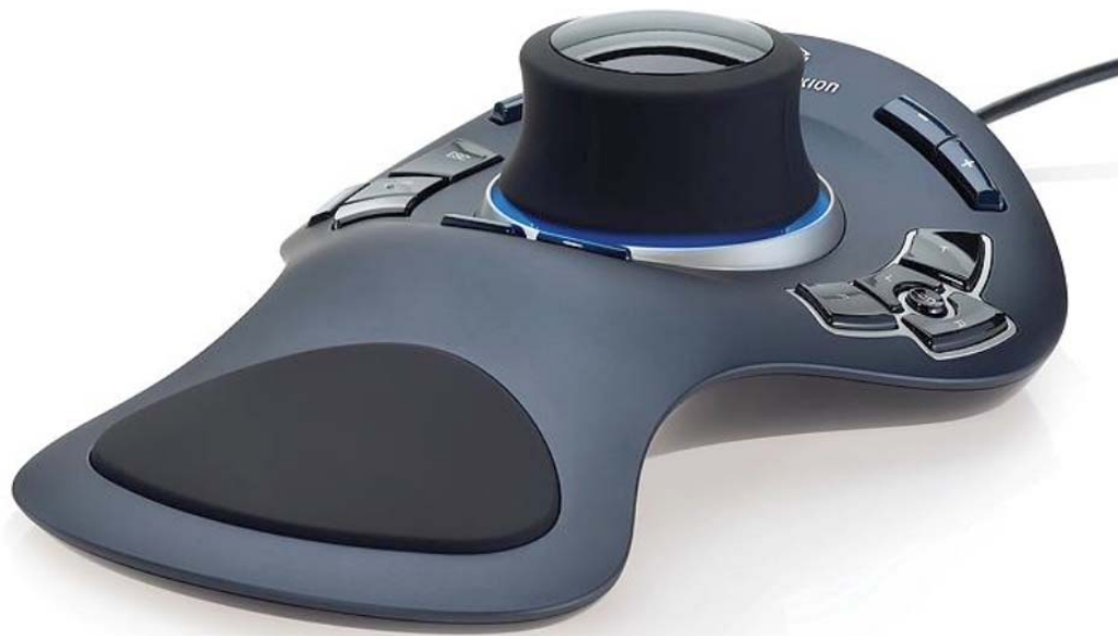
Figure 15-2: Connexion SpaceExplorer with 6 DOF Control Movement.
