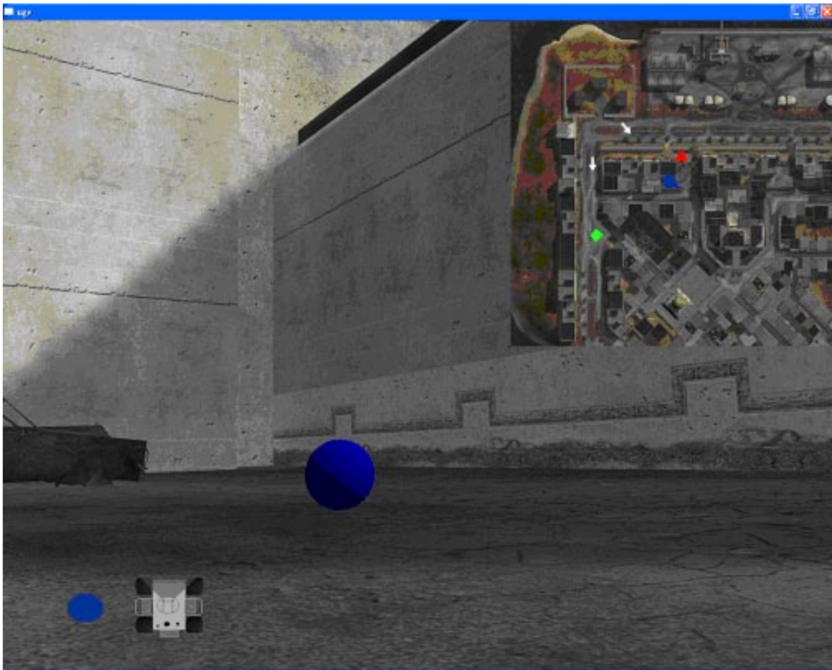
Figure 11-1: Example of the Operator's Control Station. The task was to navigate the blue UGV to the blue inspection point, the red UGV to red inspection point, and the green UGV to the green inspection as indicated on the map in the upper right corner.
