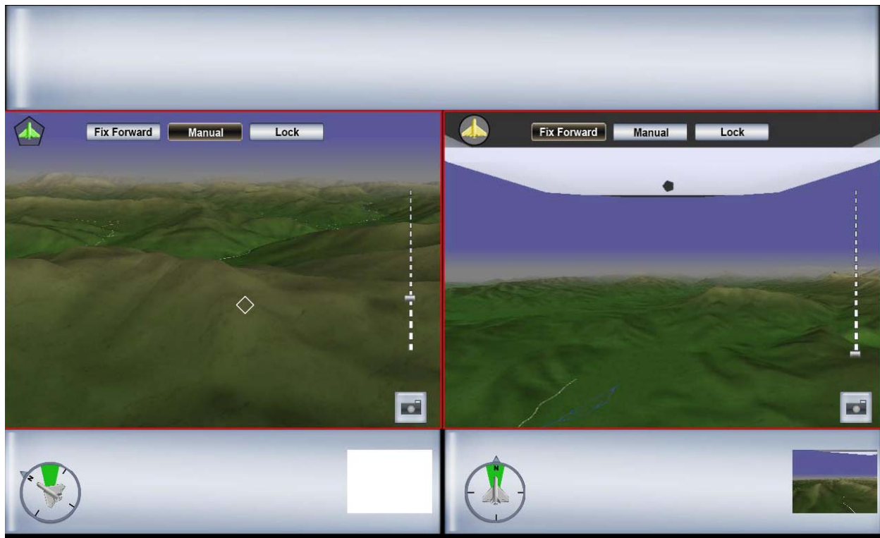
Figure 7-3: Tactical PO's Camera Views Screen.
