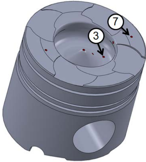
Figure 4 Piston top view showing fast response surface thermocouples
