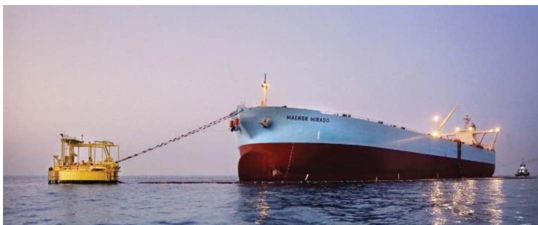
Tanker berthed at new SPM off al-Faw peninsula. (Leighton Offshore Photo.)
