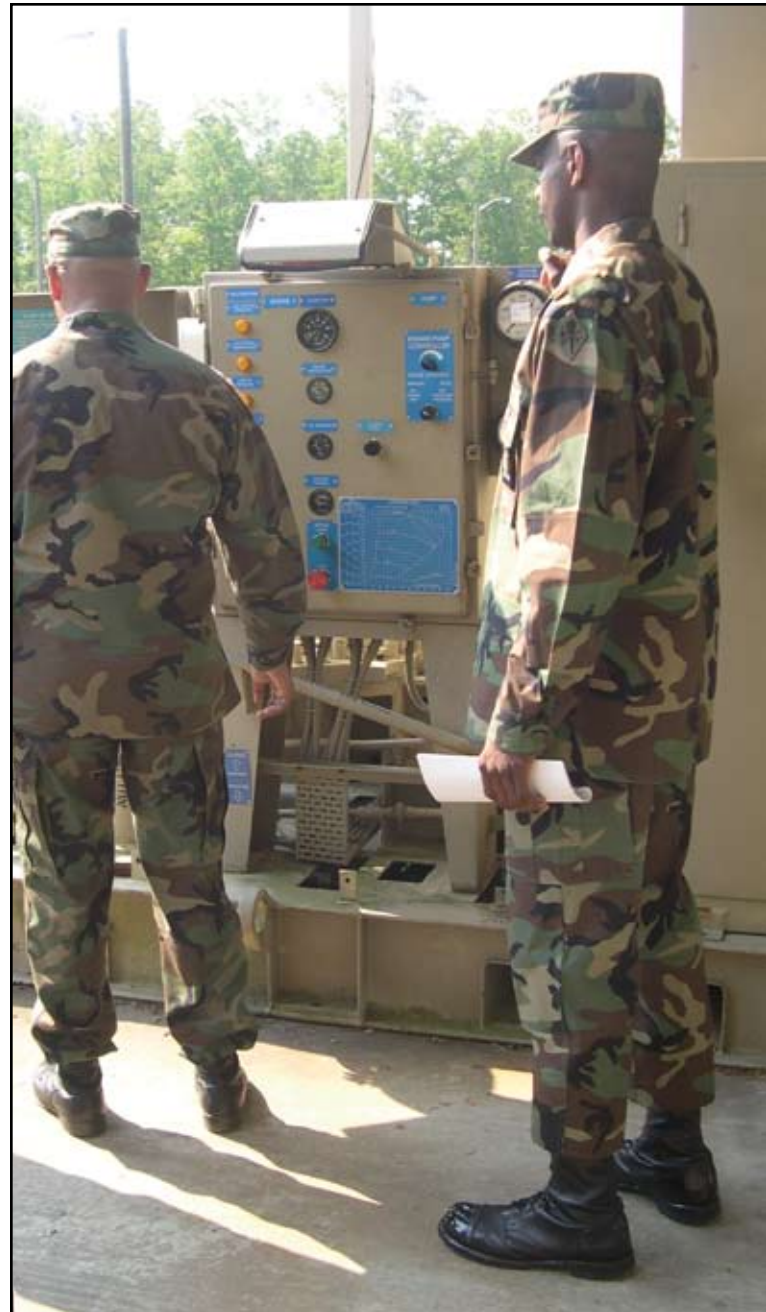
At an Inland Petroleum Distribution System site, Soldiers inventory components of an 800-gallon-per-minute mainline pump.
