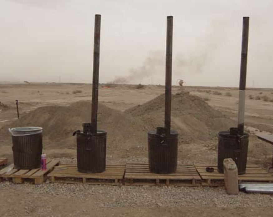
Immersion heaters (above) provide hot water for food preparation and showers (at right) in the field.
