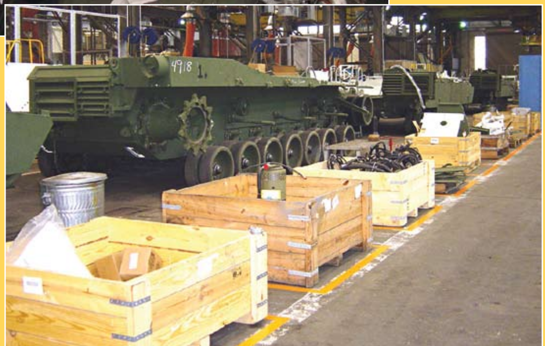
One of Anniston Army Depot's major Lean Six Sigma success stories is the M1 Abrams tank assembly line. Workers went from a bay-style operation (above) to a one-piece flow operation (at right), which reduced throughput time by 56 percent (from 4.5 to 2 days).
