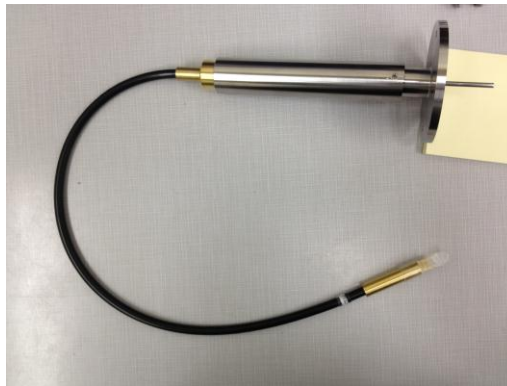
Figure 20. Scintillation-collection fiber-bundle to be integrated with the streak-camera.
