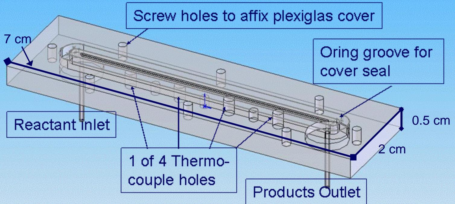
Note – reactor is sealed with a plexiglas cover for imaging abilities
