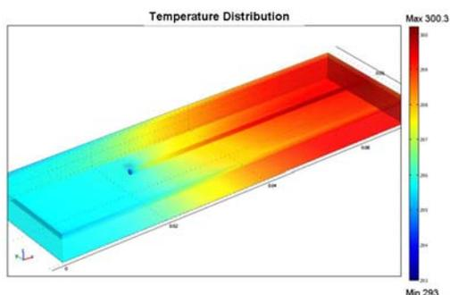
**Figure 4.** Three dimensional temperature distribution using an initial volumetric flow rate of  $2e^{-9}$  m<sup>3</sup>/s of 50% w/w H<sub>2</sub>O<sub>2</sub> over the convectively cooled microreactor.
