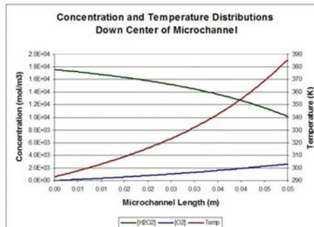
**Figure 2.** Temperature, and  $\text{H}_2\text{O}_2$  and  $\text{O}_2$  concentration distributions using an initial volumetric flow rate of  $2 \times 10^{-9} \text{ m}^3/\text{s}$  of 50% w/w  $\text{H}_2\text{O}_2$  down the center of the directly convectively cooled microchannel.
