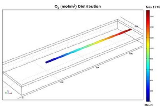
**Figure 6.** Three dimensional O<sub>2</sub> concentration distribution using an initial volumetric flow rate of  $2e^{-9}$  m<sup>3</sup>/s of 50% w/w H<sub>2</sub>O<sub>2</sub> over the convectively cooled microreactor.
