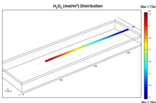
**Figure 5.** Three dimensional H<sub>2</sub>O<sub>2</sub> concentration distribution using an initial volumetric flow rate of  $2e^{-9}$  m<sup>3</sup>/s of 50% w/w H<sub>2</sub>O<sub>2</sub> over the convectively cooled microreactor.
