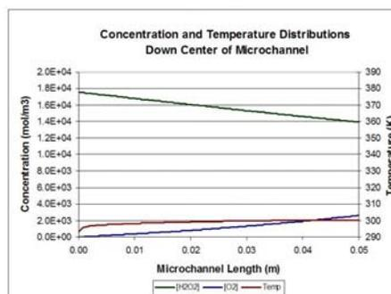
**Figure 3.** Temperature, and  $\text{H}_2\text{O}_2$  and  $\text{O}_2$  concentration distributions using an initial volumetric flow rate of  $2 \times 10^{-9} \text{ m}^3/\text{s}$  of 50% w/w  $\text{H}_2\text{O}_2$  down the center of the microchannel including the convectively cooled extended surface area.
