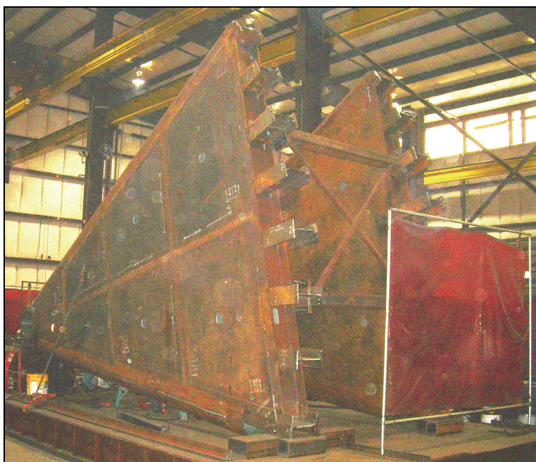
Figure 6. New John Day Lock culvert valve during fabrication.
