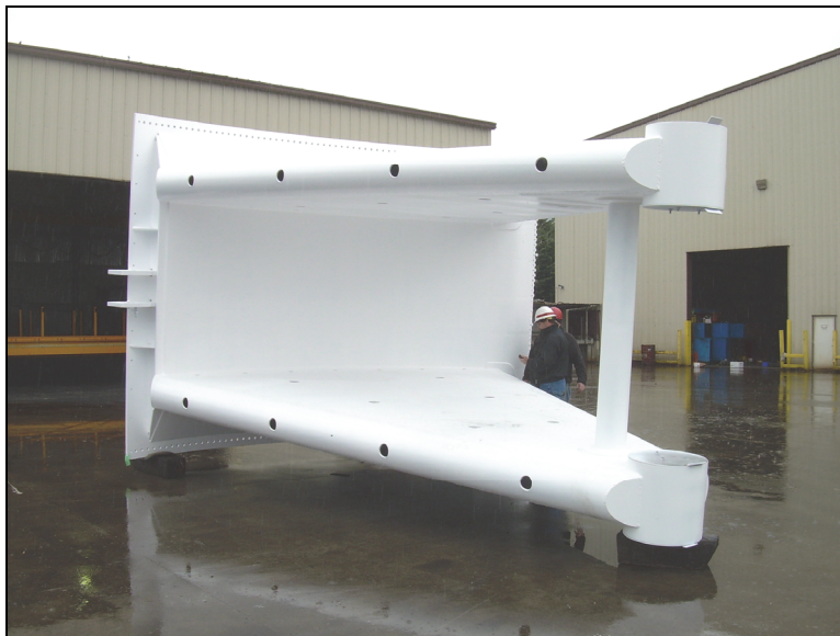
Figure 7. Newly fabricated John Day Lock culvert valve, turned on its side (top is on left).
