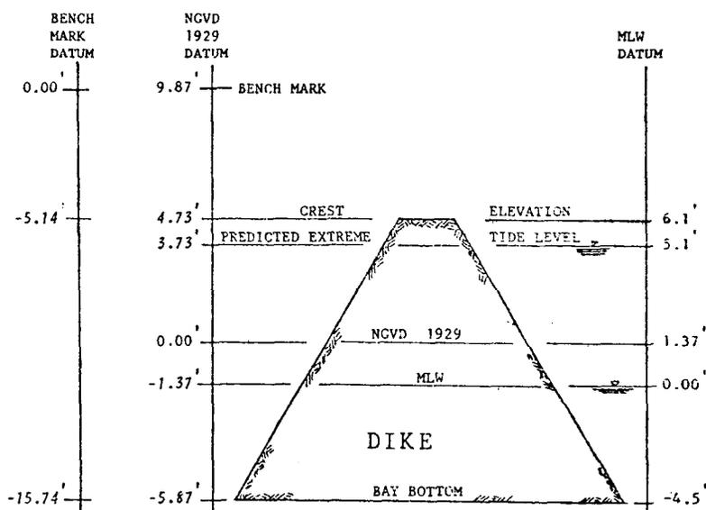
The resulting elevations are shown in italics in the figure under NGVD 1929 DATUM (which includes the land-based bench mark). The final step is to adjust the crest and toe elevations relative to the bench mark, which is taken as the zero reference.
