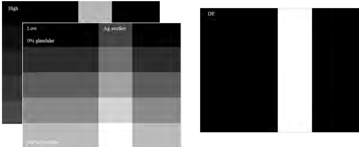
Figure 4. High (26 keV)- and Low (21 keV)- energy images of a step phantom with an section of embedded Ag. The images are subtracted using the pre-calculated weighting factor to yield the DE image shown on the right.
