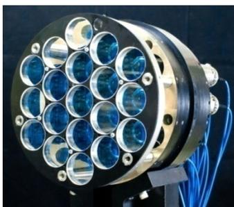
Figure 23: 19 Sub-Aperture System Built by Optonicus
