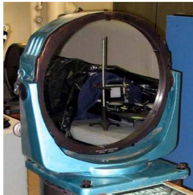
Figure 2: 24 inch (~61 cm) Mirror Used in Compact Range
