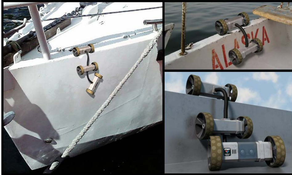
Figure 1. Conceptual MSM robot climbing hull surfaces.
