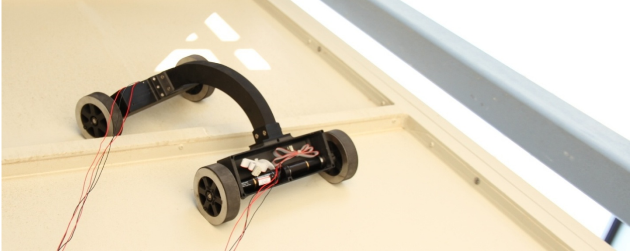
Figure 16. Prototype robot with flux-plate wheels.
