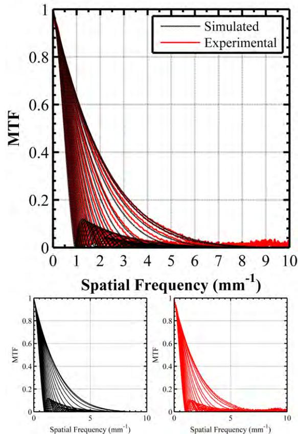
**Figure 16:** (top) The results of the analytical model of the MTF (red) superimposed against an actual MTF dataset acquired from the test tool (black), both over a range of reconstruction slice offsets from 0 to 1.9 mm in 0.1 mm steps with  $\pm 16^\circ$  angular range.
