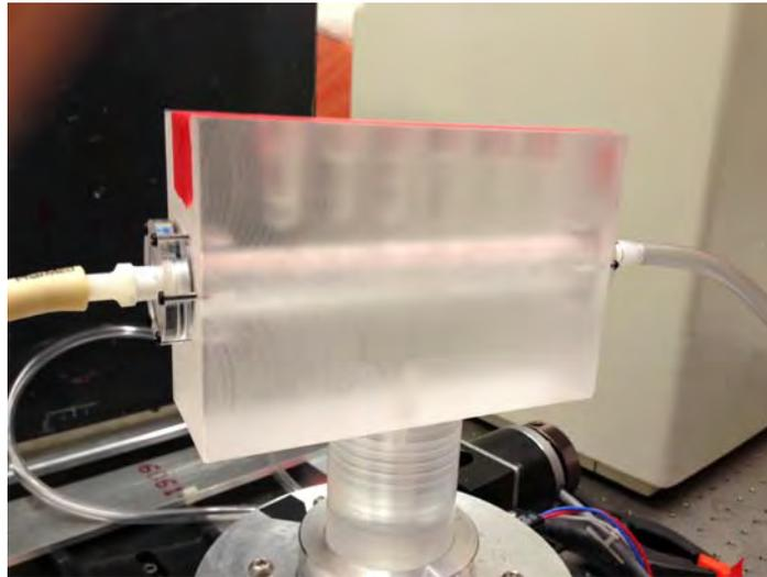
**Figure 5:** A flow phantom was built to simulate temporal dependencies of blood flow in the breast. The phantom consists of a main flow chamber connected to a pump and liquid reservoir. Contrast agent can be added to the reservoir via a power injector (not shown). Six calibration chambers are aligned along the top edge of the phantom.
