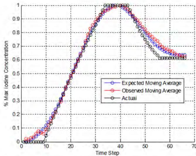
**Figure 6:** A sample temporal measurement of blood flow conducted with the imaging system. The actual iodine concentration is shown (black), together with the expected value (blue) calculated as the moving average of the actual data, and the measured results (red). Close agreement between expected and observed results is seen.
