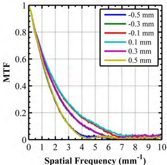
420 **Figure 15:** MTF versus frequency at different reconstruction slice depths with a reconstruction created from 9 projections and an angular range of  $\pm 16^\circ$ . It can be observed that the decay of the MTF is very similar to that seen in a reconstruction with the same angular range but more projections. The reconstruction slice offset is increased as the curves transition from superior to inferior.
