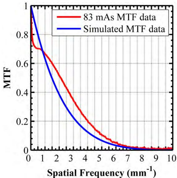
290 **Figure 6:** Simulated MTF data at 0 mm slice offset superimposed with actual 83 mAs MTF data at 0 mm slice offset. A low frequency artifact is visible in the actual data, as well as some offset in the corresponding MTF values.
