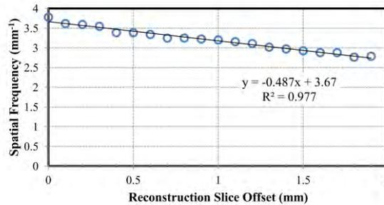
**Figure 19:** Reconstruction slice offset versus spatial frequency at which the MTF drops
