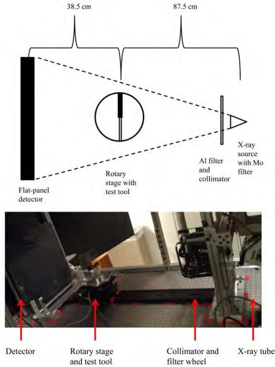
155 **Figure 2:** (top) The upper image depicts a schematic of custom x-ray imaging station from aerial view. An x-ray source, aluminum filter, and rotary stage with test object are positioned in succession in front of a flat panel detector. (bottom) The image below is a photograph of the x-ray testing station (filter wheel is not visible).
