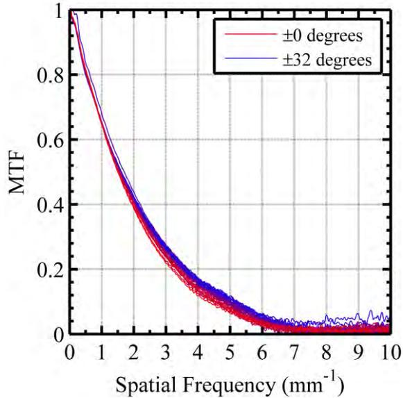
365 **Figure 11:** MTF versus frequency for a range of reconstruction slice angles in which the lead edge is positioned in the plane for each reconstruction. The MTF curves transition from blue to red as the obliquity of the reconstruction slice angle increases. A clear trend is visible that shows the MTF degrading slightly as the obliquity increases (from the superior to the inferior curves).
