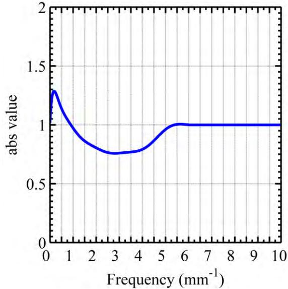
300 **Figure 7:** The quotient of the simulated MTF with no slice offset and the actual MTF
