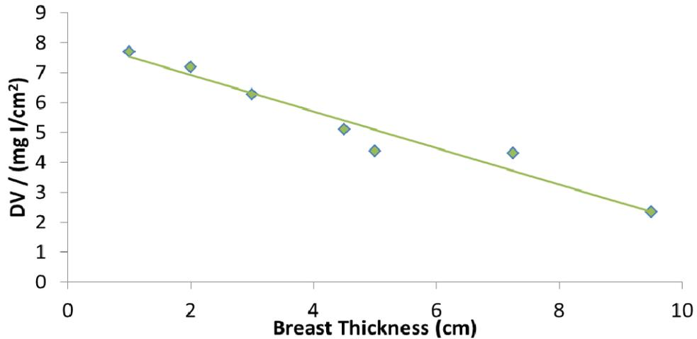
**Figure 4.** (a) Using static phantoms of different thickness, it is possible to quantify the signal as a function of areal density. Two thicknesses are shown for illustration. (b) The calibration coefficient (slope of lines in Fig 4a) can then be calculated for each breast thickness.
