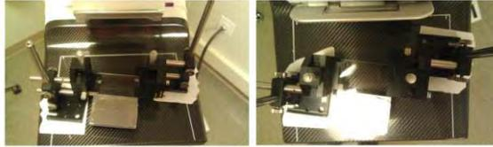
320 **Figure 8:** Experimental setup to measure MTF in planes offset from the plane of the lead
