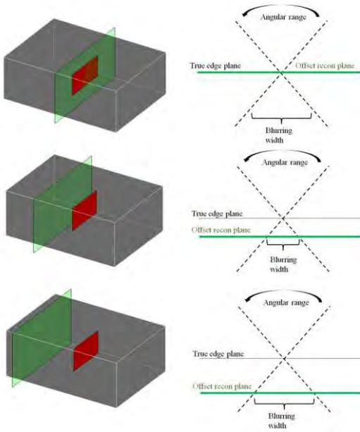
200 **Figure 4:** (left) Graphical depiction of the process by which the MTF is analyzed at each increasing reconstruction slice offset, in which a feature of interest is in the smaller (red) plane and the reconstruction plane is shown as the larger (green) plane. (right) Graphical depiction of the intersection of the projections at the plane containing a feature of interest and the reconstruction plane.
