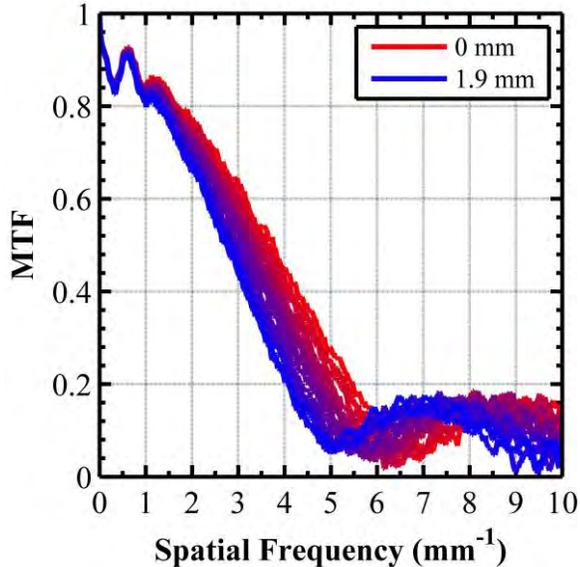
465 **Figure 18:** MTF versus frequency in Hologic tomosynthesis reconstructions where the lead edge is moved away from the reconstruction slice that contains the edge. The MTF can be seen to decay as the slice moves further from the slice containing the edge (as the curves transition from superior, red, to inferior, blue).
