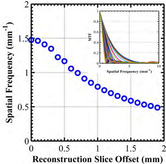
350 **Figure 10:** The spatial frequency at which the MTF drops to 50% of its maximum value versus the reconstruction slice offset over a 0-2 mm range of slice offsets, in 0.1 mm increments. The pictograph in the upper right corner shows the original MTF data for this set of reconstruction slice offsets.
