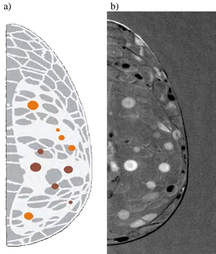
**Figure 3.** (a) A schematic diagram showing one layer of the contrast phantom. The inclusions are specified in Table 1. (b) A hybrid temporal dual-energy subtraction radiograph of the phantom showing the iodine inclusions.
