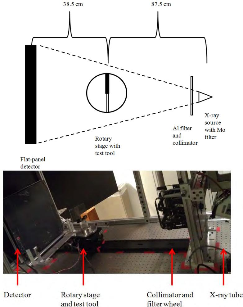
**Figure 2:** (top) The upper image depicts a schematic of custom x-ray imaging station from aerial view. An x-ray source, aluminum filter, and rotary stage with test object are positioned in succession in front of a flat panel detector. (bottom) The image below is a photograph of the x-ray testing station (filter wheel is not visible).
