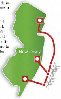
The first phase of the project will be the New Jersey Energy Link, which is capable of carrying 3,000 megawatts of offshore wind and delivering it to the strongest points on the terrestrial grid.
