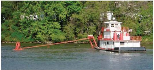
The UTV *Misty Dawn* the afternoon of April 18, 2010, shortly after the barge it had been pushing sank. The photo clearly portrays the minimal freeboard of the vessel and the two open doors along the port side of the vessel leading into the main engine and equipment spaces. All factors, combined with lack of watertight integrity, contributed significantly to the rapid progressive flooding of the main spaces and the subsequent sinking of the vessel later that night. U.S. Coast Guard photo.
