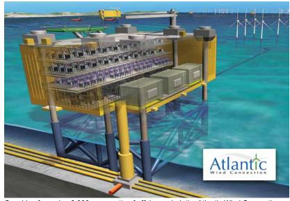
Capable of carrying 6,000 megawatts of offshore wind, the Atlantic Wind Connection project is designed to increase the reliability and efficiency of the existing land-based electrical grid. All graphics courtesy of the Atlantic Wind Connection.
