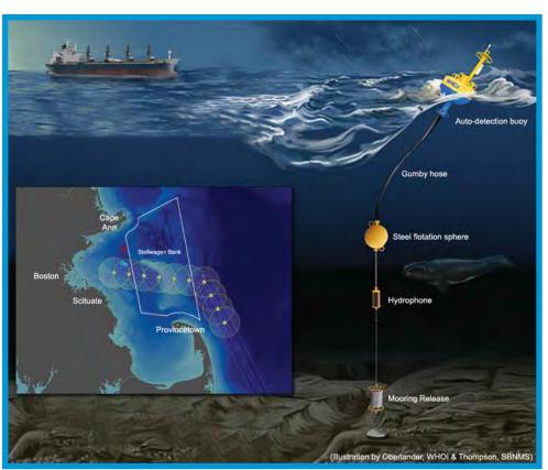
Buoys detect the presence of a right whale through the whale's "up call," and use a satellite connection to relay the call spectrogram to scientists for species confirmation. LNG companies paid for the acoustic detection system as part of their USCG and MARAD licensing agreements. Illustration by E. Paul Oberlander, Woods Hole Oceanographic Institution, and graphic adapted courtesy of NOAA/Stellewagen Bank National Marine Sanctuary.
