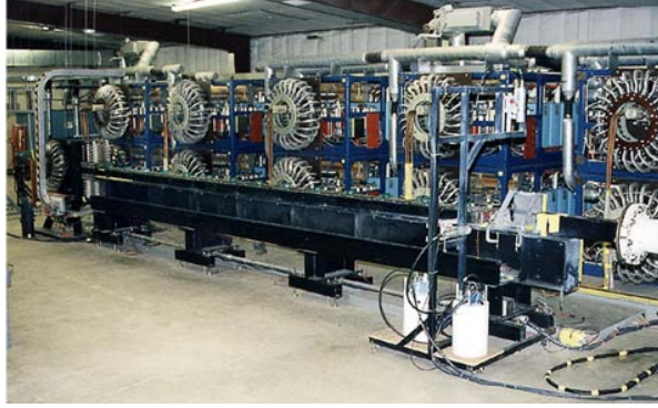
Figure 1-2. UT-IAT's electromagnetic launch facility (ELF).
