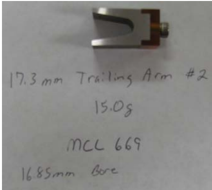
Figure 2-24. Photograph of a solid armature with robust trailing arms.
