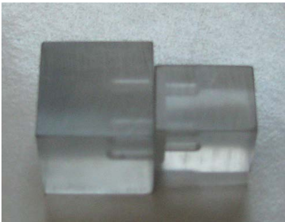
Figure 2-6. Carrier and projectile coupled together before a shot.
