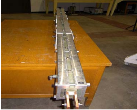
Figure 3-7. Assembled breech-fed launcher.
