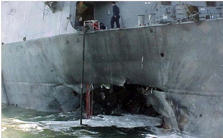
Figure 5. Damage to the USS Cole from a WBIED Attack (From Sutton, 2011)
