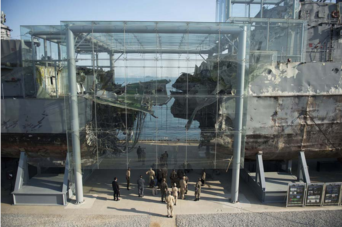
Figure 4. Damage to the Cheonan from a Torpedo Detonation (From CNO Visits ROKS Cheonan Memorial, 2013)
