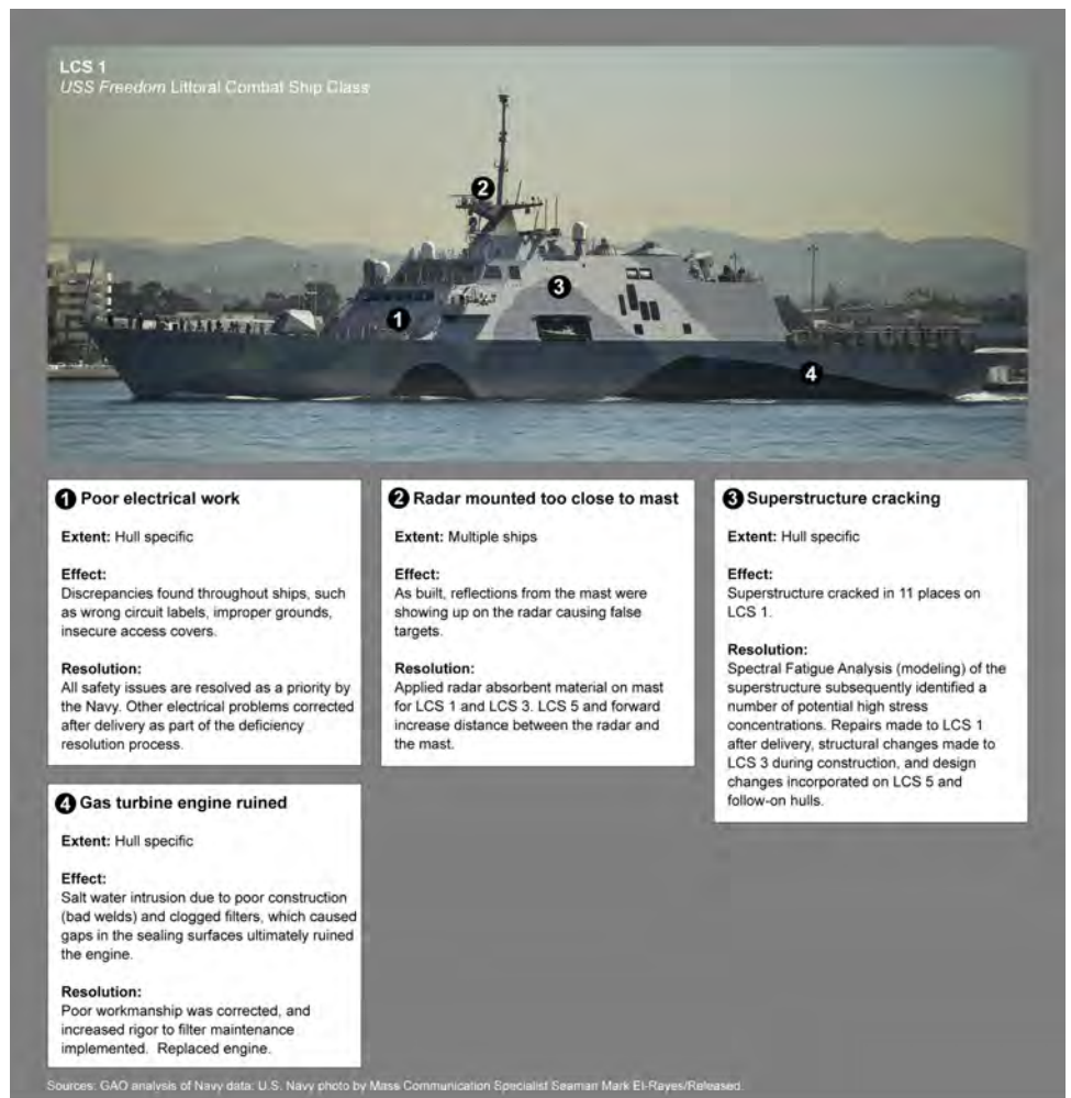
Figure 18: Selected Quality Issues on USS Freedom (LCS 1)
