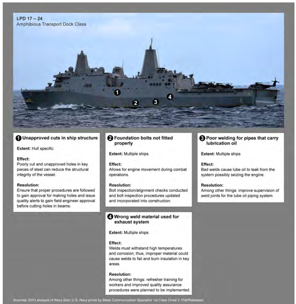
Figure 21: Selected Quality Issues on LDP 17 Class Ships
