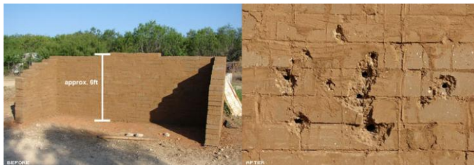
Figure 25. CEB ballistics test specimens (Leading Edge Group, Inc.).
