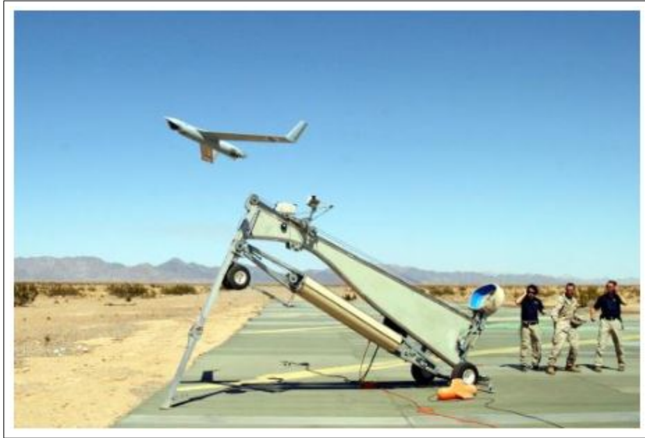
Figure 2.4: Scan Eagle and launch system. From [10]
