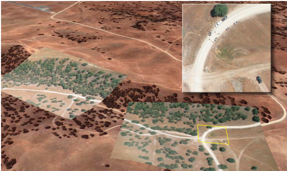
Figure 11. Sample photographs automatically placed over background imagery and terrain using only recorded telemetry for position. The inset photo illustrates the level of detail afforded by the system.
