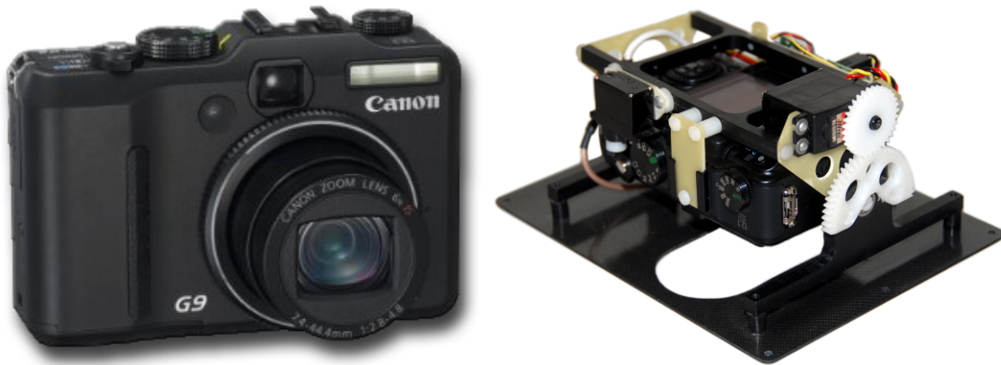
Figure 9. Canon G9 camera and roll-axis gimbal mount providing +/- 45 degree of roll compensation and side-look pointing.
