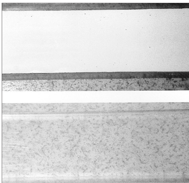
Figure 4: Polycarbonate annular reactor coupons used in the biofilm prevention study; the coupons contain the biocidal polyurethane coating (top) and no coating (bottom)
