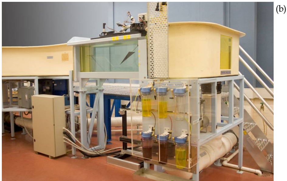
Figure 3. Eidetics Model 1520 water tunnel; (a) diagrammatic view of tunnel, (b) photograph of tunnel.
