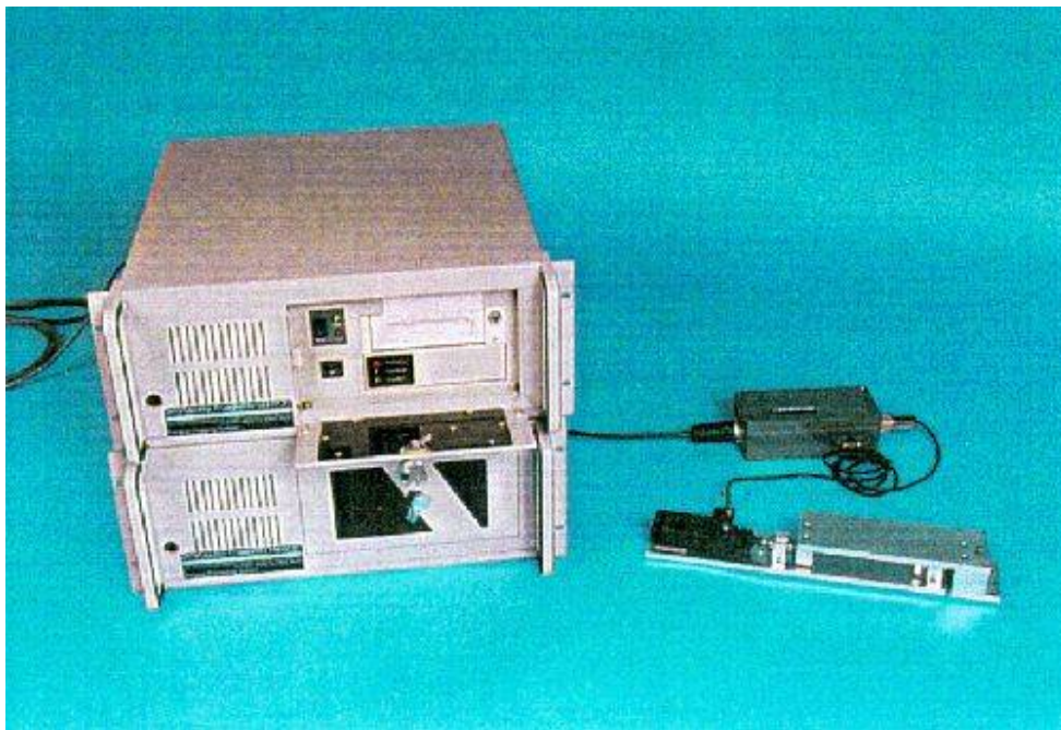
Figure 5. DERA wave induced fatigue strain recorder with one optical strain gauge.
