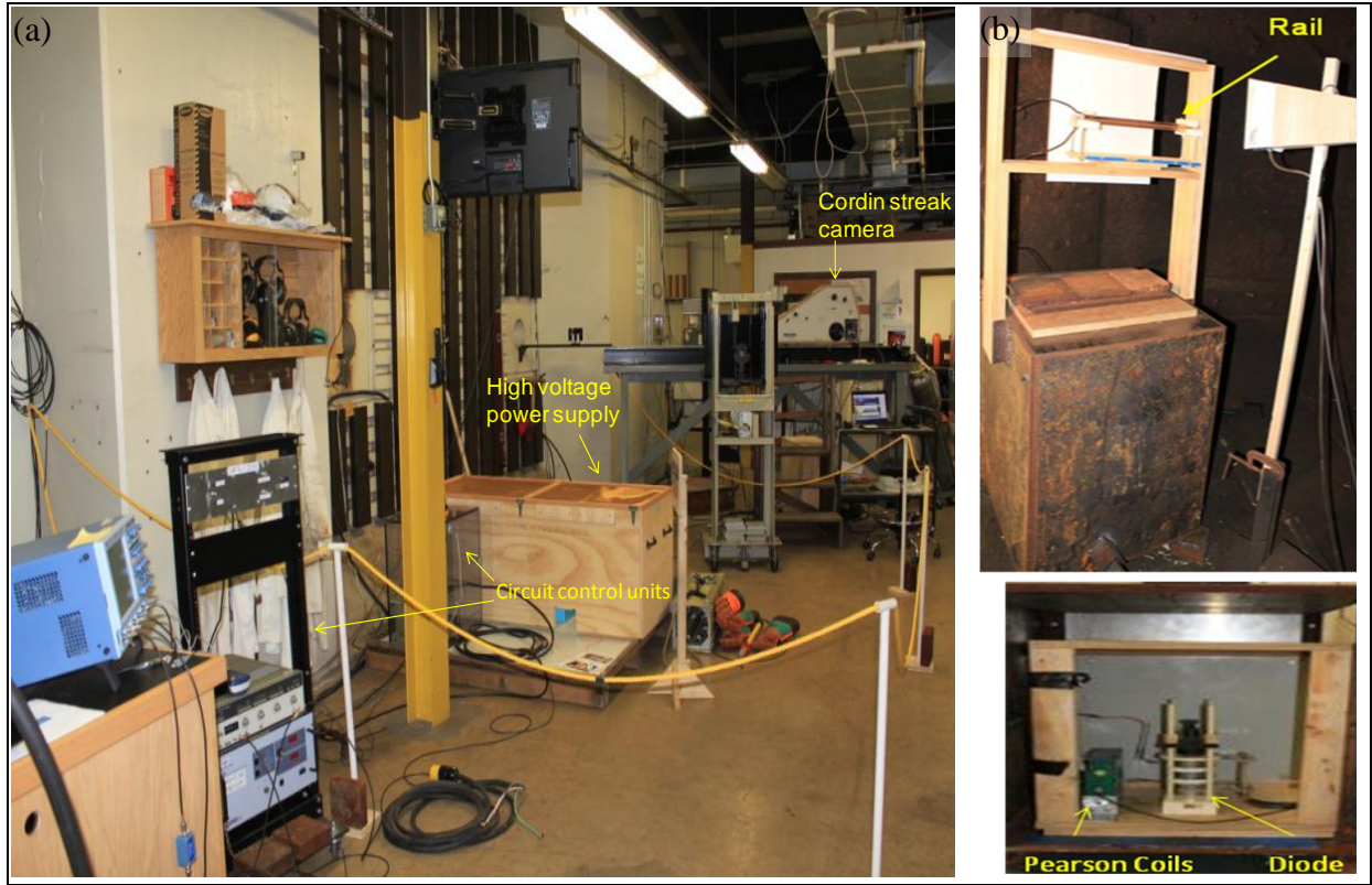
Figure 6. Experimental arrangement (a) outside the blast chamber and (b) inside the blast chamber.
