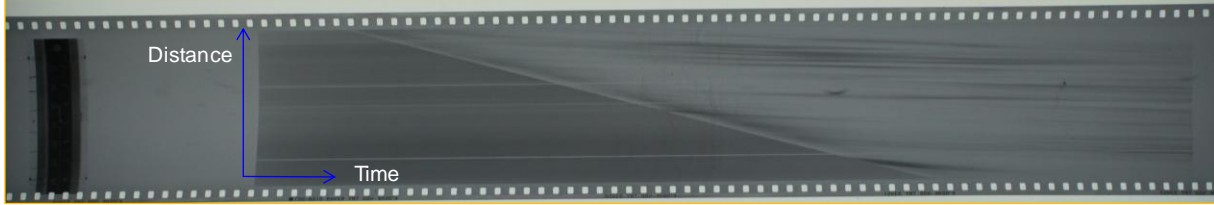
Figure 13. A typical streak record with an electric energy input of 160.33 kJ.
