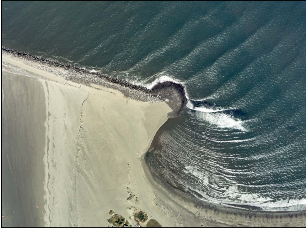
Figure 11. Mound diffraction structure as constructed at Grays Harbor, WA (2000)
