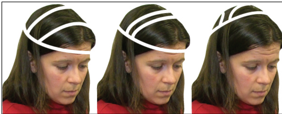
Figure 3. Three potential attachment configurations. Left: general EEG set-up with sensors distributed across the head. Middle: central configuration for maximal sensor coverage over the motor cortex which could be used for motor control applications. Right: posterior configuration with maximal sensor coverage over the occipital cortex, which could be used for visual detection applications.
