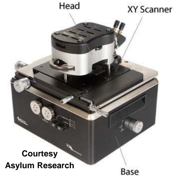
Multi-frequency AFM to study mechanical dissipation as a function of temperature (Local Thermal Analysis)
