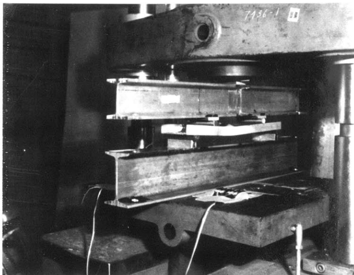
FIG. 8: SANDWICH BEAM 3 IN TEST JIG AFTER FAILURE
