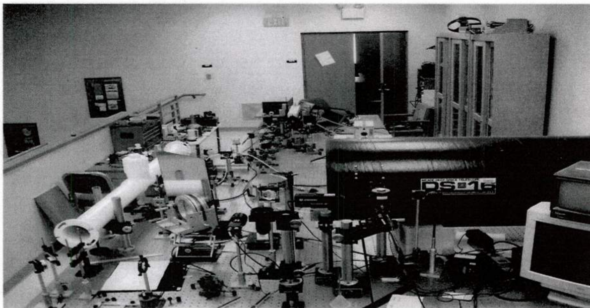
Figure 5. (a) Upper Photo: Gold coated retro reflector array; (b) lower photo: photograph of laboratory CO 2 laser DIAL system
