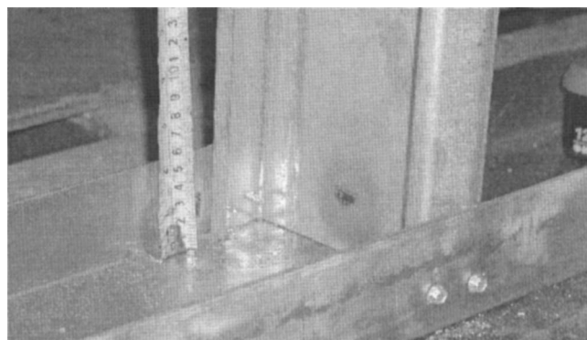
Fig. 5. Bottom stud-to-track connection using two #10 TEK screws for W3 and W4
