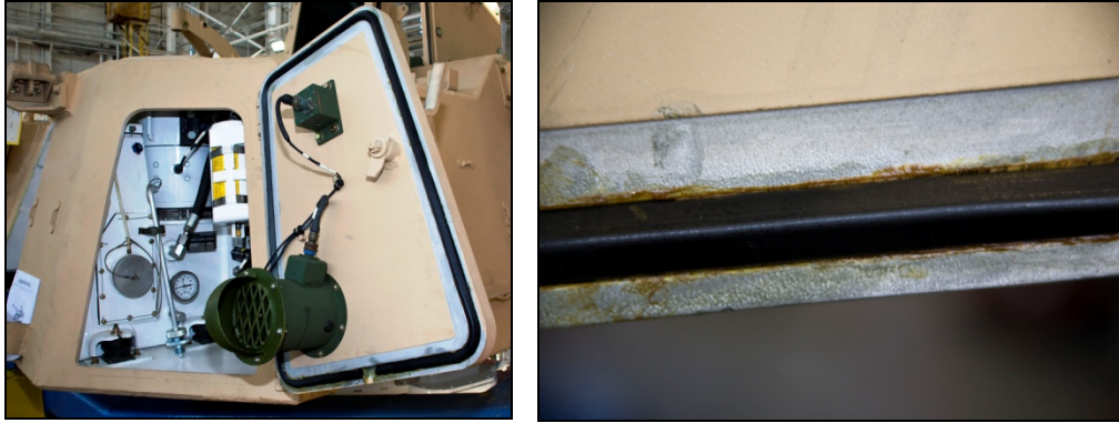
Figure 6. Bonded gasket on hydraulic compartment hatch door.
