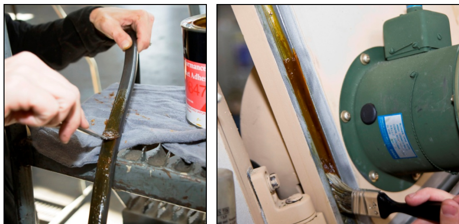
Figure 5. Adhesive application on rubber seal (left) and aluminum channel (right).
