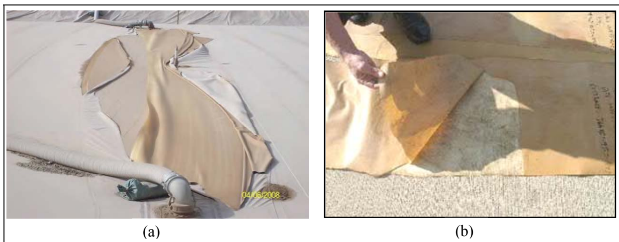
Figure 2. (a) Fabric delaminations of inservice fuel storage tanks and (b) large coating to fabric bonding failure due to surface fuel pooling and leaching.
