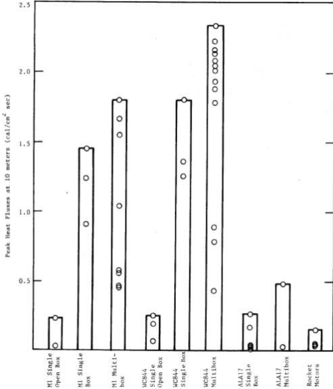
FIGURE 146. Comparison of Heat Fluxes (Figure 34 From Reference 43) [1 cal/cm²sec = 41.868 kW/m²].
