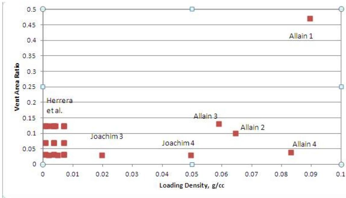
FIGURE 162. Plot of Loading Density vs. Area Ratio for Tests.
