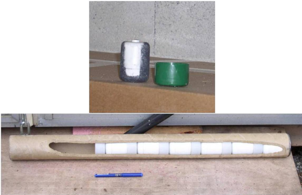
FIGURE 102. Light Effect Shell Containing Stars and Bursting Charge and Cutaway of a Candle Showing Shells and Lifting Charges.
