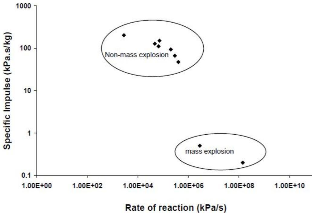
FIGURE 115. Relationship Between Maximum Rate of Reaction (Maximum  $Dp/Dt$ ) and Specific Impulse ( $I_s^{10-90}$ ) for a Range of Packaged Fireworks.
