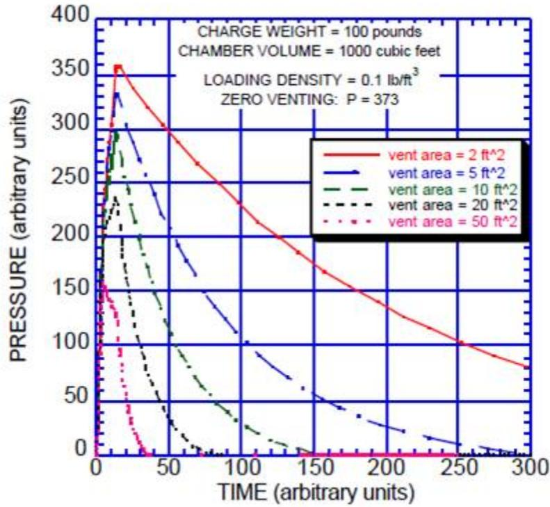
FIGURE 183. Pressure–Time for Various Amounts of Venting and 100 Pounds Burning (Reference 53).
