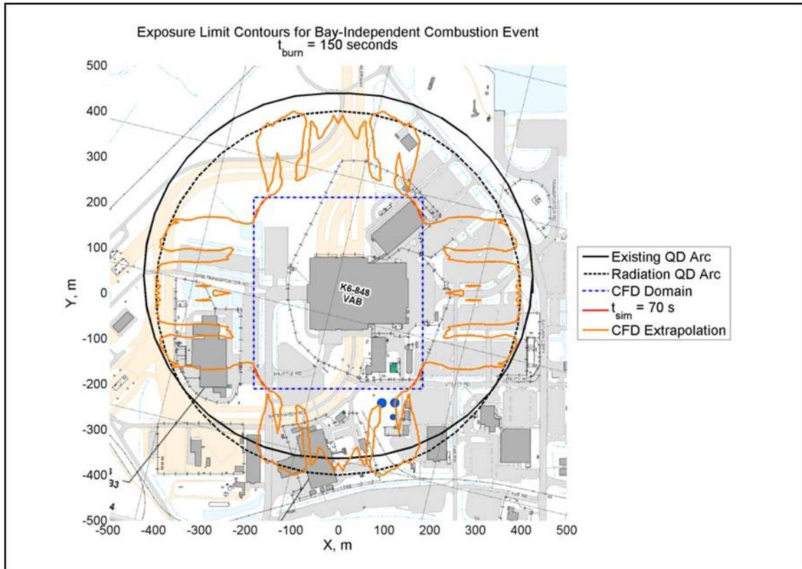
FIGURE 200. Contour Map Showing One Region Where Safe-Separation Distances, Using Radiation Method, Were Slightly Outside Arc Determined for SSP (Reference 45).
