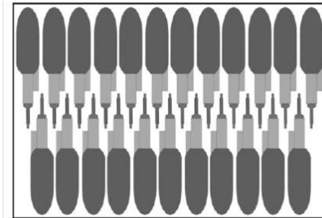
FIGURE 113. Packing Arrangement for Each Layer of WP6 Stickless Rockets. Each layer of stickless rockets separated with a layer of cardboard.
