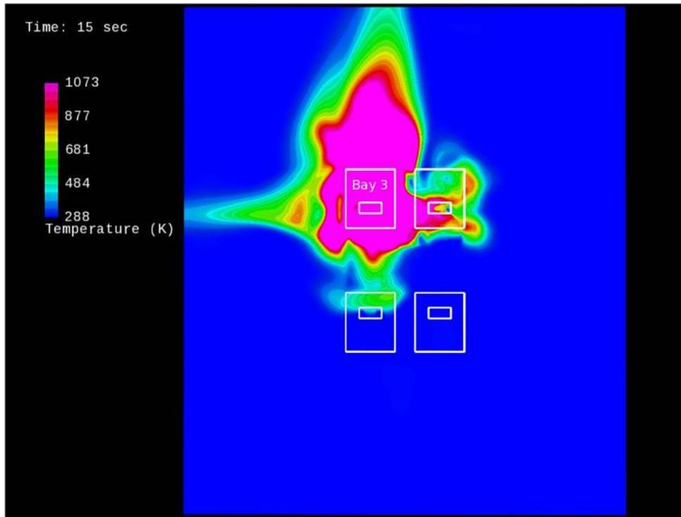
FIGURE 194. Temperatures of Exhaust Plumes at 1.68 Meters (66 Inches) Above the VAB Floor 15 Seconds After Ignition of Boosters in High Bay 3 for Scenario 1d (Reference 45).
