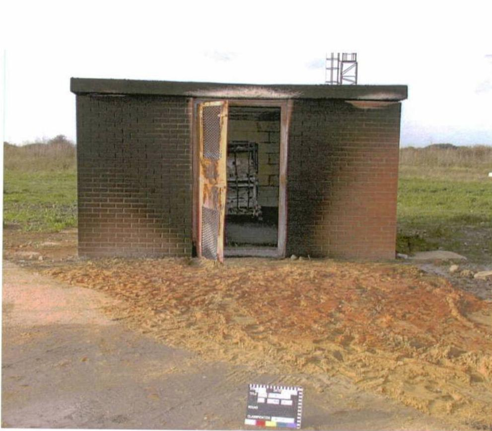
FIGURE 165. Results of the Tests With 155-mm Propelling Charges Subjected to Standard Liquid Fuel Fire Within Building (Reference 50).
