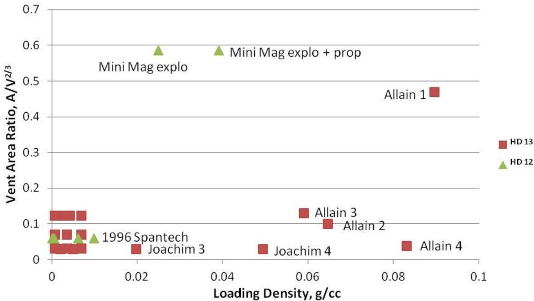
FIGURE 181. Plot of Vent Area Ratio and Loading Density for Various Tests.
