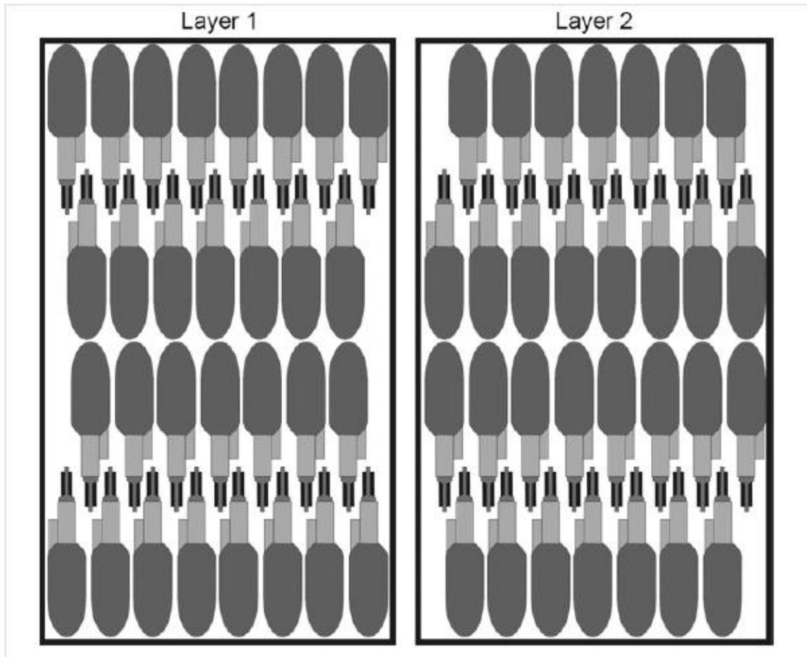
FIGURE 114. Packing Arrangement for Two Layers of WP 9 Stickless Rockets, With No Cardboard Separating Layers.
