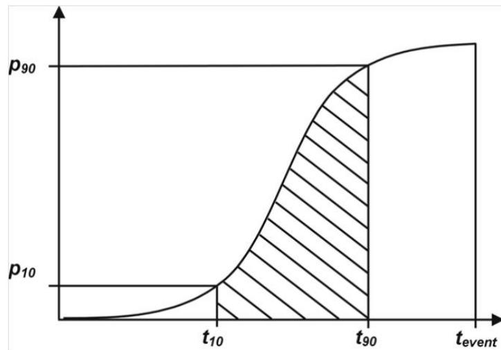
FIGURE 112. Portion of the p-t Curve Used to Calculate the Specific Impulse.
