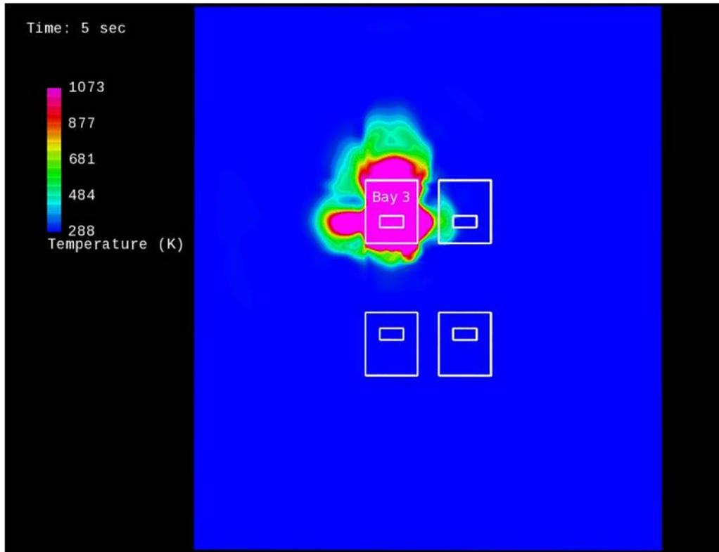
FIGURE 193. Plan View of Temperatures of Exhaust Plumes at 1.68 Meters (66 Inches) Above the VAB Floor 5 Seconds After Ignition of Boosters in High Bay 3 for Scenario 1d (Reference 45).
