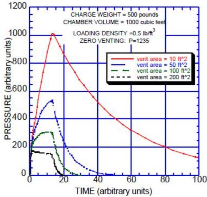
FIGURE 184. Pressure–Time With Various Amounts of Venting for 500 Pounds Burning (Reference 53).
