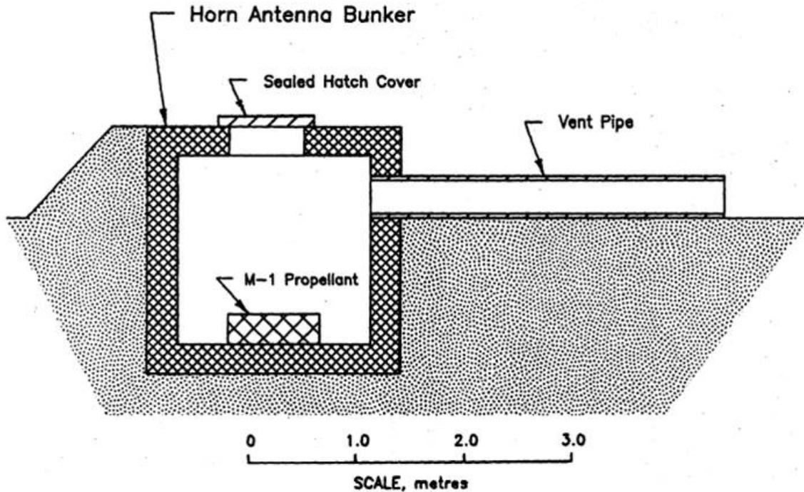
FIGURE 151. Schematic of Test Chamber and Vent Pipe (Reference 47).
