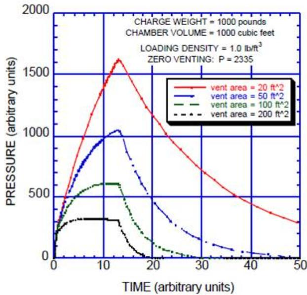
FIGURE 185. Pressure–Time With Various Amounts of Venting for 1,000 Pounds Burning (Reference 53).
