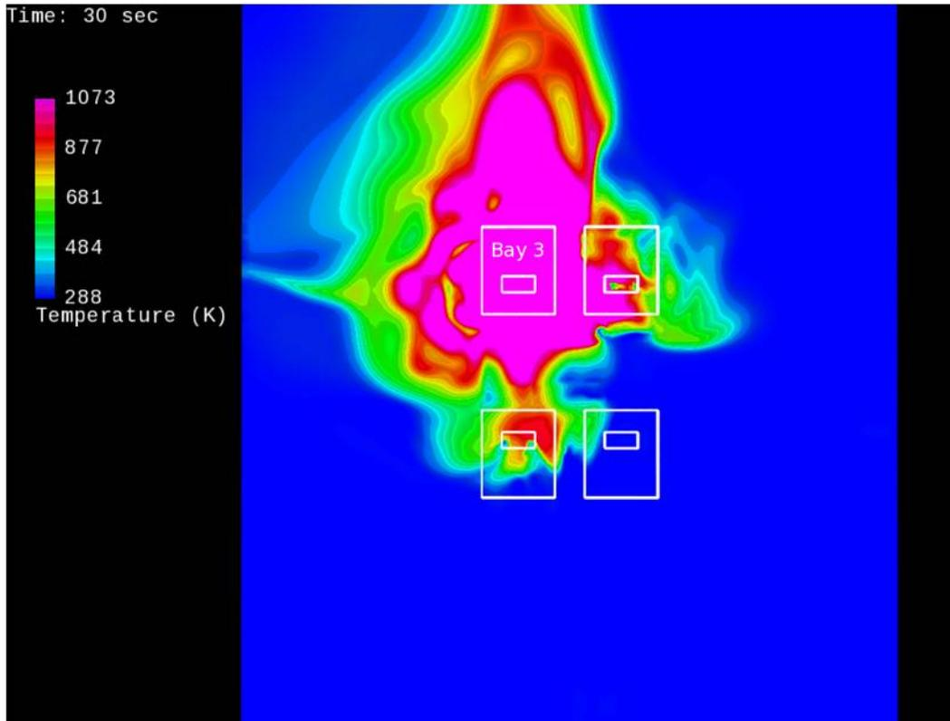
FIGURE 195. Temperatures of Exhaust Plumes at 1.68 Meters (66 Inches) Above the VAB Floor 30 Seconds After Ignition of Boosters in High Bay 3 for Scenario 1d (Reference 45).
