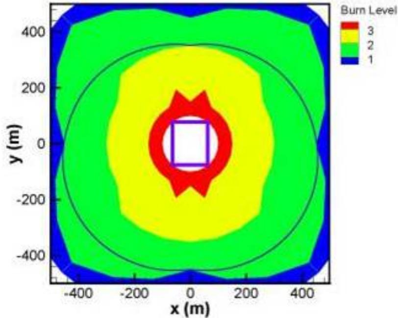
FIGURE 198. Scenario 1d Contour Map of Burn Level Due to Radiation as a Function of Position Around VAB for One Motor Pair (Burning in Same Bay) (Including Safety Factor and Solar Isolation) as Determined Using FDS Code (Reference 45).
