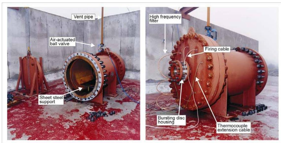
FIGURE 111. Pressure Vessel Used in WP8.
