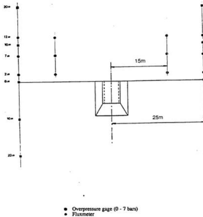
FIGURE 157. Location of Flux Sensors 2, 7, and 12 m x 15 and 25 m and Overpressure Gauges at 0, +20 m, and -20 m by 25 m (Reference 48).
