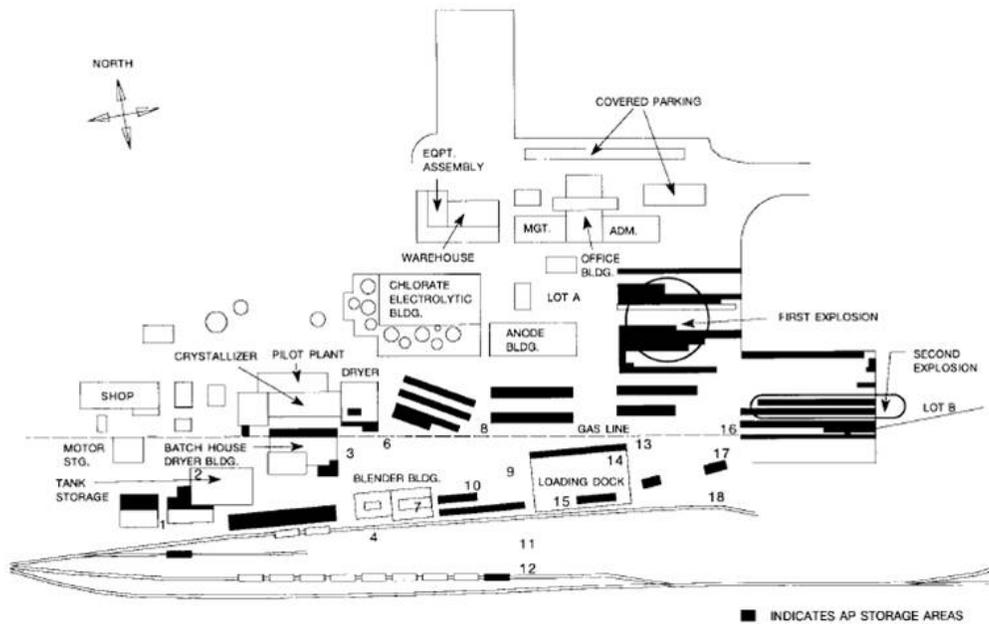
FIGURE 136. Mapping of the PEPCON Facility Showing the Buildings and AP Storage Areas (Reference 37).
