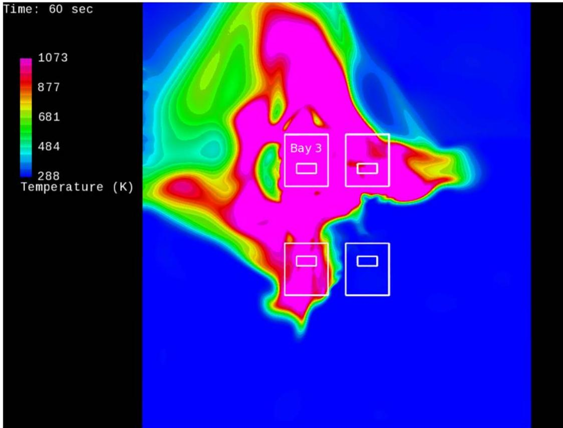
FIGURE 196. Temperatures of Exhaust Plumes at 1.68 Meters (66 Inches) Above the VAB Floor 60 Seconds After Ignition of Boosters in High Bay 3 for Scenario 1d (Reference 45).
