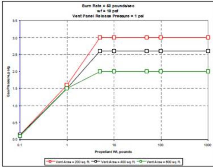
FIGURE 189. Pressure Variation With Vent Area (Figure 6 of Reference 67).
