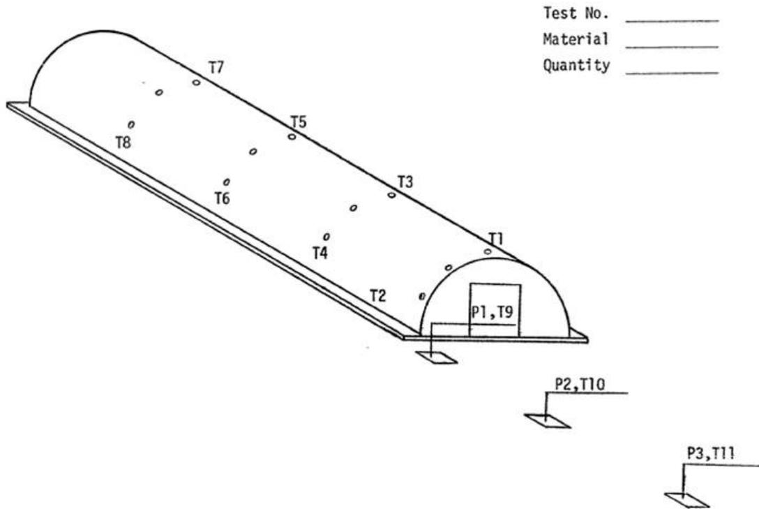
FIGURE 148. Schematic of 1/10th Scale Igloo With Sensors/Location.
