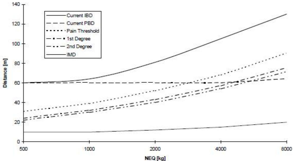
FIGURE 201. Results of Lawton's Calculations for Open Burning of Propellant MNLF2P Compared to Current Inhabited Building Distance IBD and Process Building Distance PBD.
