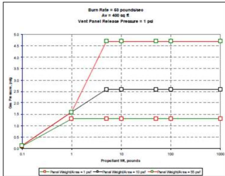
FIGURE 190. Pressure Variation With Panel Weight/Area (Figure 7 of Reference 67).
