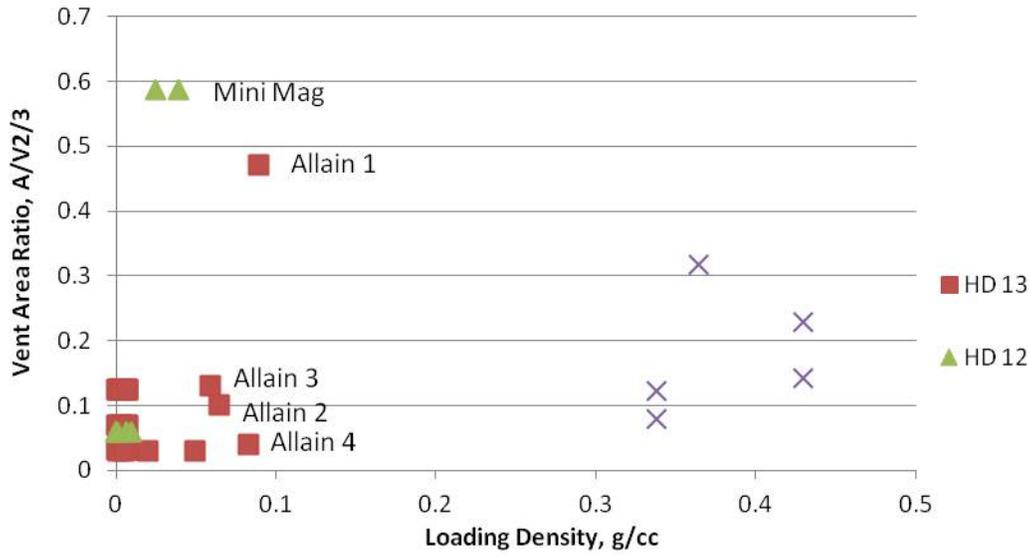
FIGURE 182. Vent Area Ratios and Maximum Loading Densities for Three of the Magazines from Table 29, With Data Points From the Previously Presented Tests. (Left to right, RC Arch 421-80-05 80 ft long and either 64 or 100 sq. ft. doors, RC Box 421-80-06, and RC Circular Arch NAVFAC with either 100 or 160 sq. ft. doors.)
