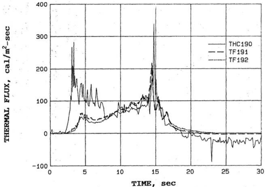
FIGURE 154. Calculated Pseudo-Thermal Flux (from Temperature Measurements of Gage (THC190) in the Bunker Chamber Compared to Measured Thermal Flux-Time Histories in the Vent Pipe (Gages TF191 and TF192) (Figure 22 From Reference 47).
