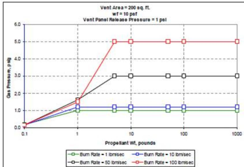
FIGURE 188. Pressure Variation With Burn Rate (Figure 5 of Reference 67).
