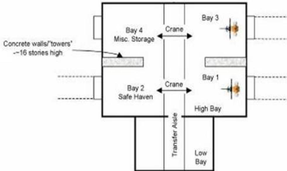
FIGURE 192. VAB High Bay and Transfer Aisle Locations.
