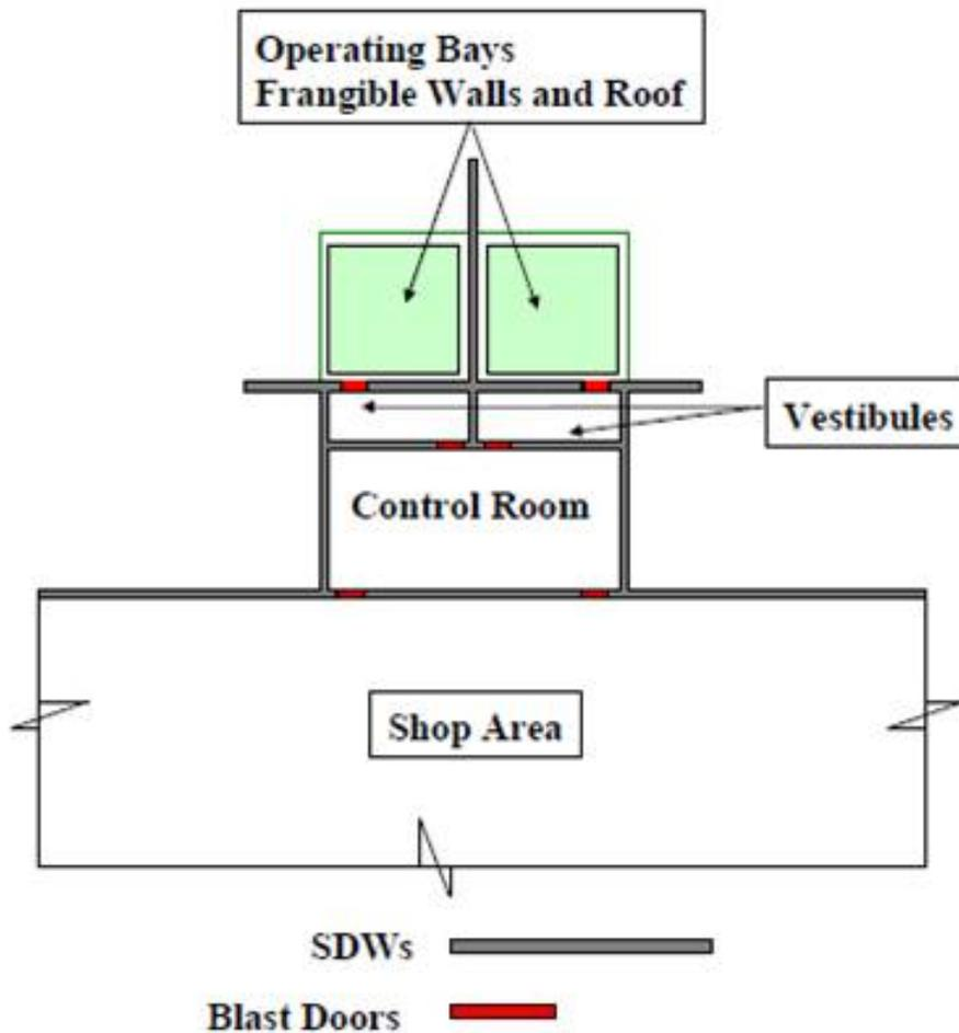
FIGURE 187. Schematic of Facility Considered in References 67 and 68.
