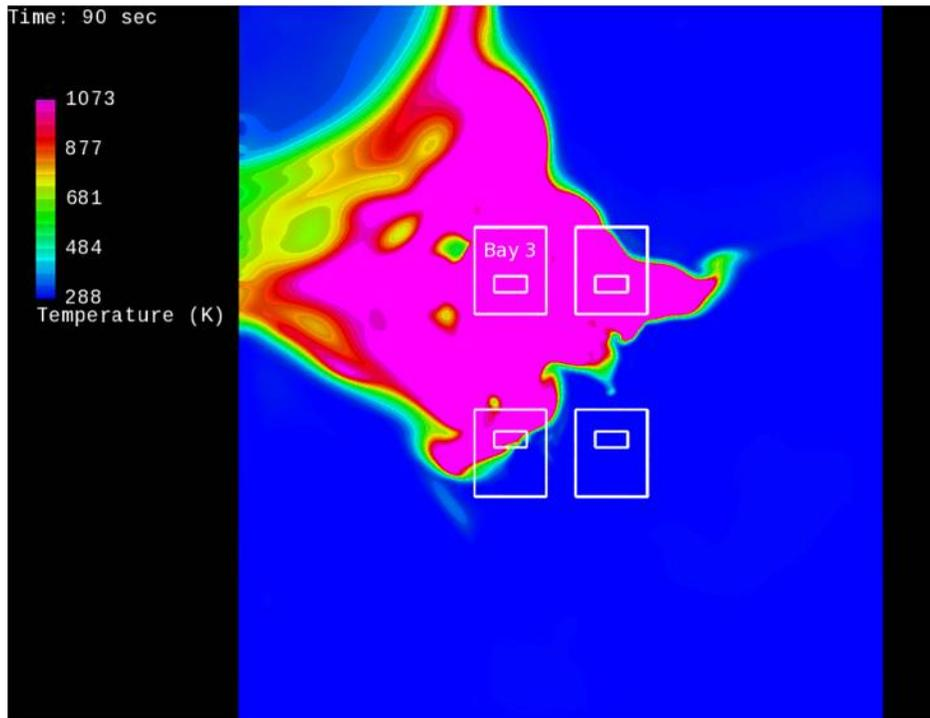
FIGURE 197. Temperatures of Exhaust Plumes at 1.68 Meters (66 Inches) Above the VAB Floor 90 Seconds After Ignition of Boosters in High Bay 3 for Scenario 1d (Reference 45).
