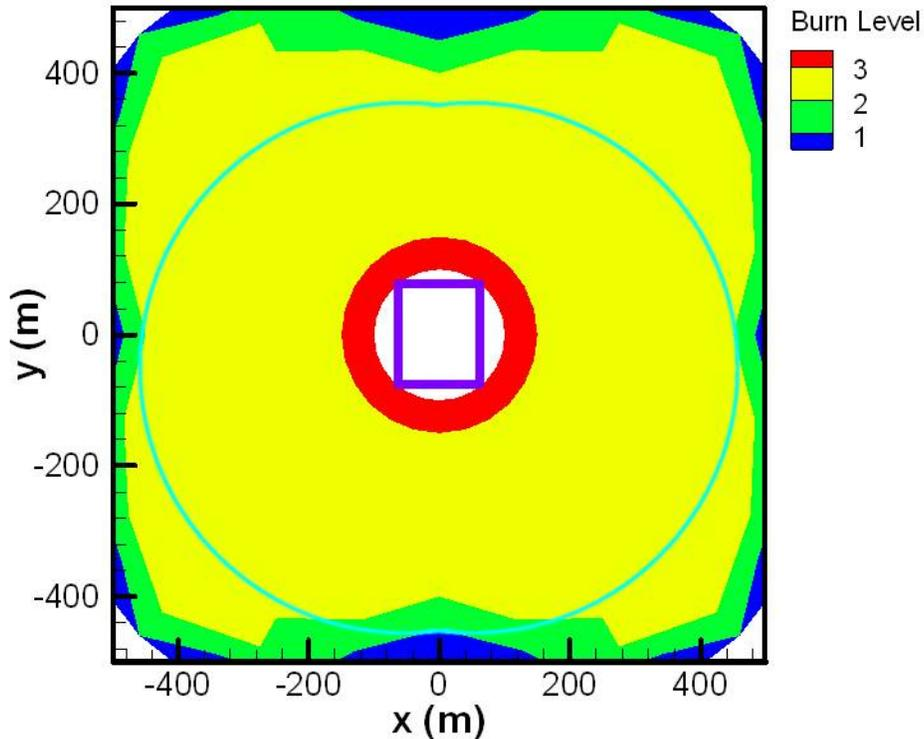
FIGURE 199. Scenario 1d Contour Map of Burn Level Due to Radiation as a Function of Position Around VAB for All Eight Boosters Burning (Including Safety Factor and Solar Isolation) as Determined Using FDS Code (Reference 45).
