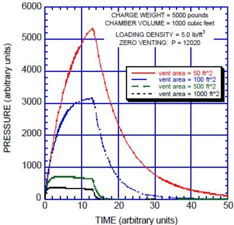
FIGURE 186. Pressure–Time for Various Amounts of Venting for 5,000 Pounds Burning (Reference 53).
