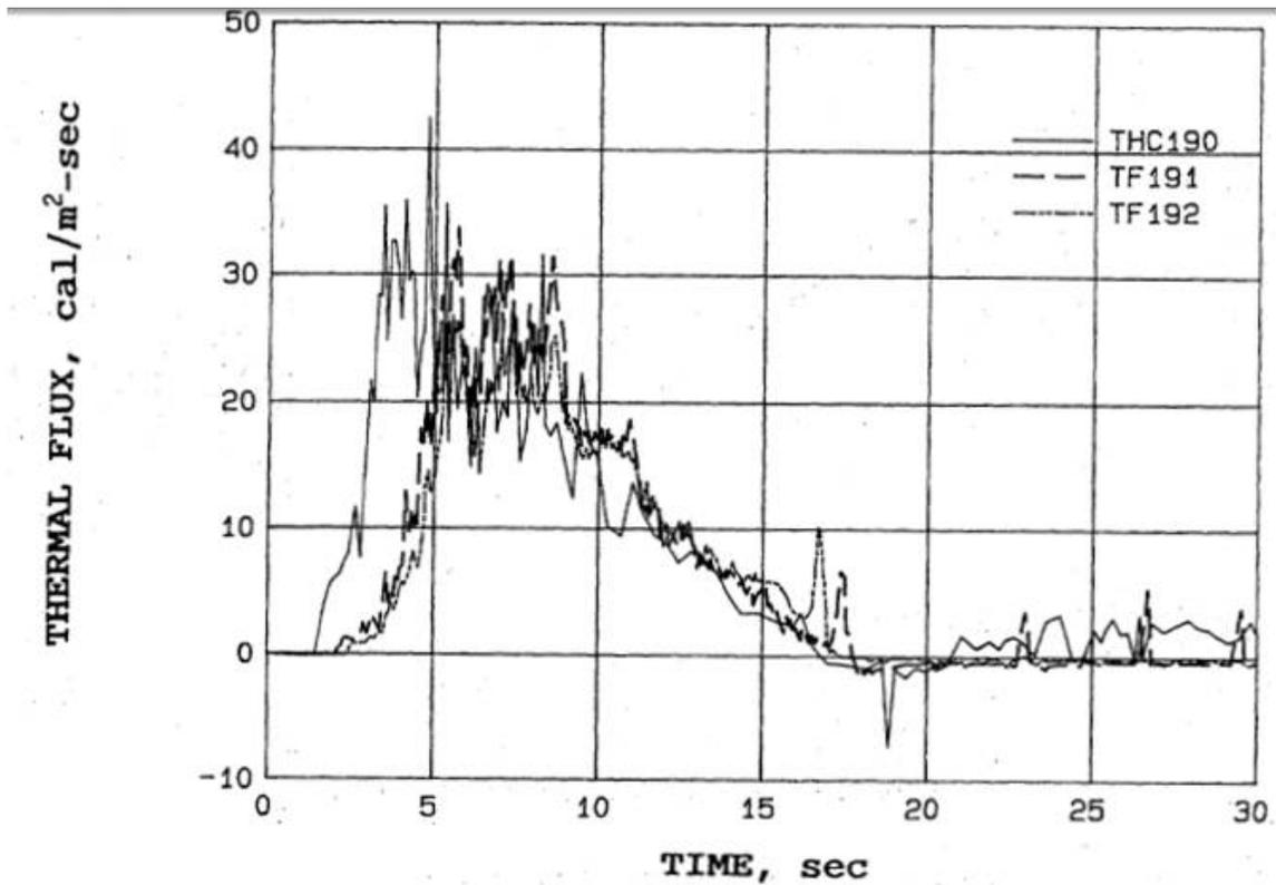
FIGURE 152. Calculated Pseudo-Thermal Flux (from Temperature Measurements of Gage (THC190) in the Bunker Chamber Compared to Measured Thermal Flux-Time Histories in the Vent Pipe (Gages TF191 and TF192) (Figure 14 of Reference 47).
