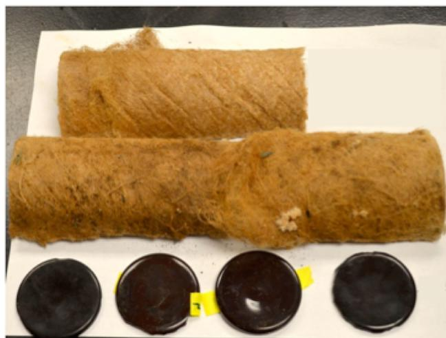
**Figure 1.** Image of a 25 cm long sediment filter and XRF disks from a home in Utility A. Filter was in use for four years.
