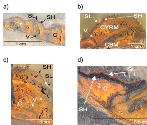
**Figure 3.** Digital images of a cross-section of representative iron corrosion products from (a) Utility A, (b) Utility B, (c) Utility C, and (d) Utility D. The C (core), CYRM (core-yellowish-red brown material), CBM (core-black material), V (veins), SH (shell layer) and SL (surface layer) are indicated in the cross-section images. The scales are in cm.
