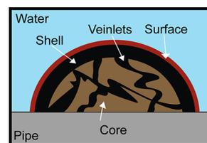
**Figure 2.** Schematic of the idealized internal structure of a mound-shaped iron drinking water pipe corrosion product (after refs 14, 21, and 47).
