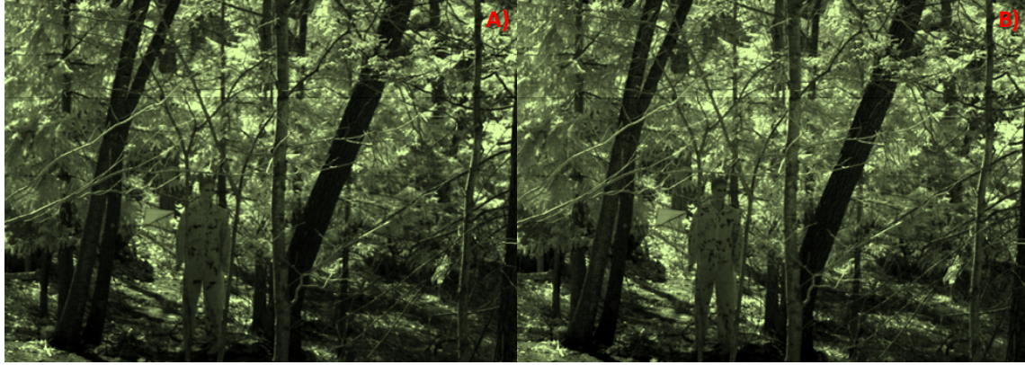
Figure 7. Green tinted monochromatic images representation for the Type 2 pattern on a jumpsuit worn by a life-sized target at (A) 780 nm and (B) 880 nm.
