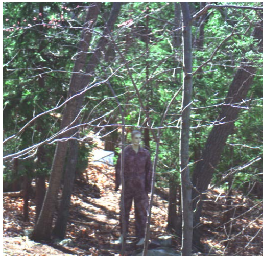
Figure 6. RGB representation for Type 2 pattern on a jumpsuit worn by a life-sized target with two NIR dyes applied (780 and 880 nm).
