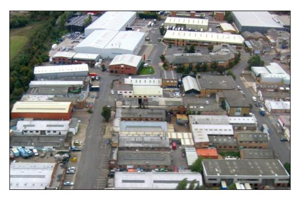
Figure 19. Most of the industrial/storage buildings in this complex have metal pitched roofs.
