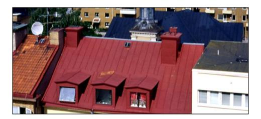
Figure 26. Ribbed steel roof (middle), tile roof (left), and rolled roofing (right) in northern Europe.
