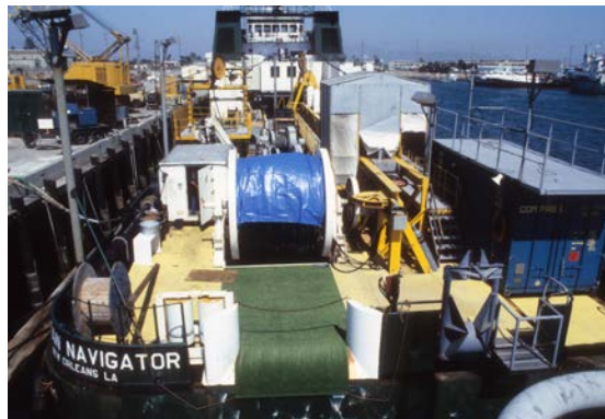
Research Vessel Acadian Navigator showing spool and winch for the towed horizontal line receiving array at dock of the Naval Civil Engineering Laboratory, Port Hueneme, California (Courtesy Dr. B.B. Adams)
