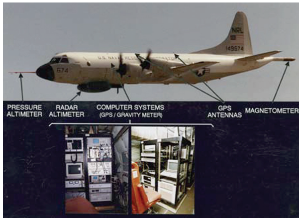
NRL airborne magnetic and gravimetric survey systems on board NRL maritime patrol aircraft (P-3).
