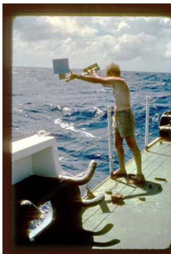
Deployment of underwater sound source with mechanical drag plate to slow its descent during direct-path scattering experiments on board HMNZS Tui in 1979 (Courtesy Dr. B.B. Adams)
