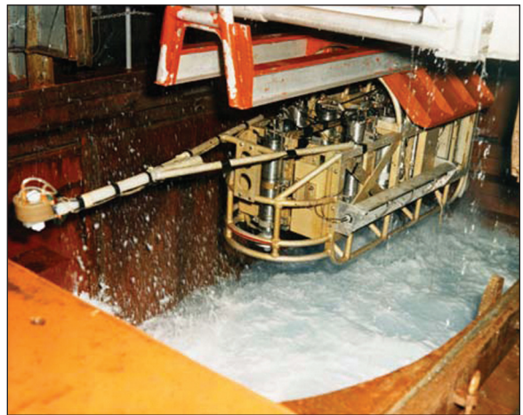
NRL instrumented towfish for deep ocean search system (mid-1960s).
