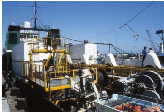
Rear deck of the Research Vessel Acadian Navigator showing the scientific equipment trailers and the five-element experimental low frequency source transducer array on its deployment track (Courtesy Dr. B.B. Adams)
