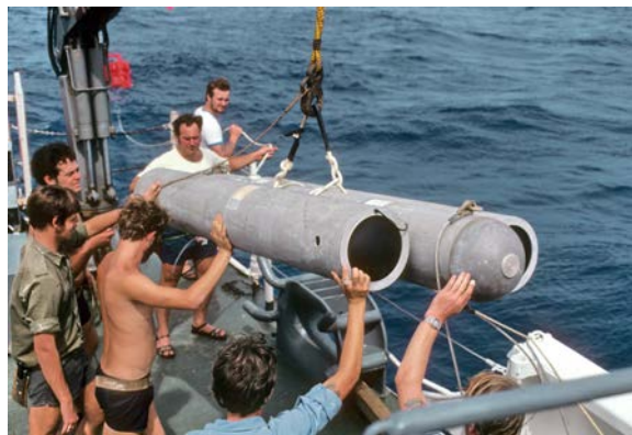
Deployment of underwater sound source transducer during NRL experiments aboard HMNZS Tui in 1979 (Courtesy Dr. B.B. Adams)
