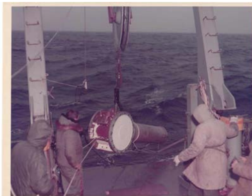
Deployment of an acoustic source transducer for Arctic transmission loss tests from fantail of USNS Mizar in 1974
