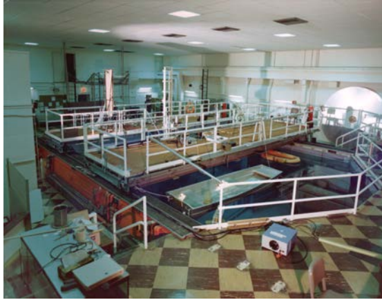
NRL's decommissioned nuclear reactor pool that was placed in use as a large acoustic test pool facility in the early 1970s (approximately 8 m x 10 m x 6 m deep at the shallowest point; with 150,000 gallons of filtered and deionized water)
