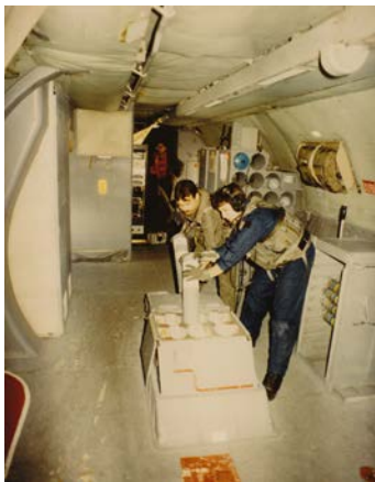
Cooperative Education trainee Matthew Fierst (center) assists Navy personnel in deployment of sonobuoys from an NRL P-3 research aircraft during an airborne sea surface scattering field experiment
