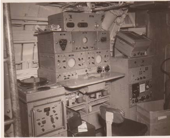
Submarine USS SeaCat SS399, XDG sonar equipment (1950)
