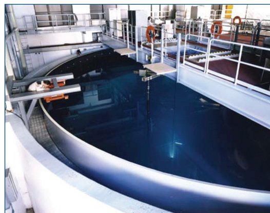
The NRL Laboratory for Structural Acoustics contains a large tank for in-water structural acoustics studies. The tank is 55 ft in diameter, 50 ft deep, and contains 800,000 gallons of deionized water.
