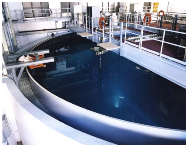
NRL Acoustics Division's Laboratory for Structural Acoustics. Large acoustic tank for in-water structural acoustics studies. It is 55 ft in diameter, 50 ft deep, and contains 800,000 gallons of deionized water.
