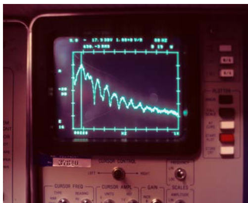
Spectrum analyzer display showing characteristic “bubble pulses” for monitoring the quality of received reverberation from impulsive source data (Courtesy Dr. B.B. Adams)
