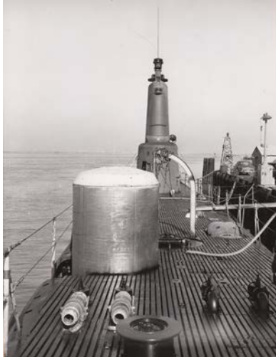
Submarine USS Guavina SS362, 10 kHz long range sonar housing (1951)
