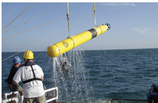
A 21-inch-diameter AUV is used for detection and classification in mine hunting and antisubmarine warfare applications.
