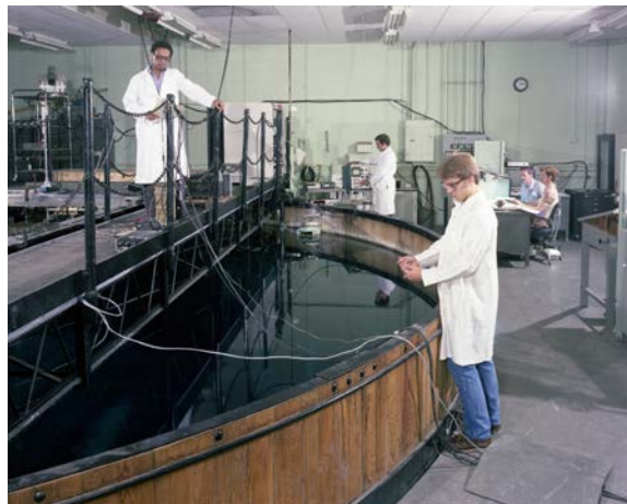
Redwood test tank (9 m diameter, 6 m deep) used for underwater scattering experiments
