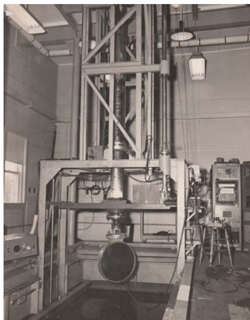
Sonar transducer testing at Dodge Pond (1950s)
