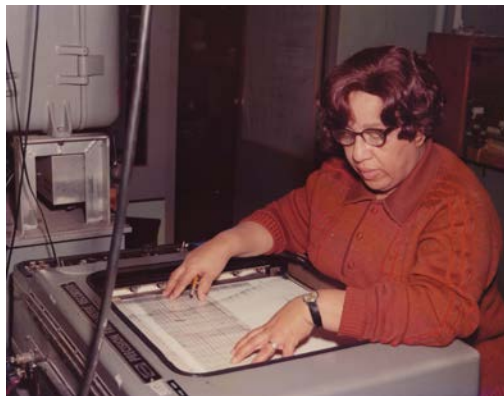
Berthel Carmichael operating a precision depth fathometer during Arctic testing aboard USNS Mizar in 1974
