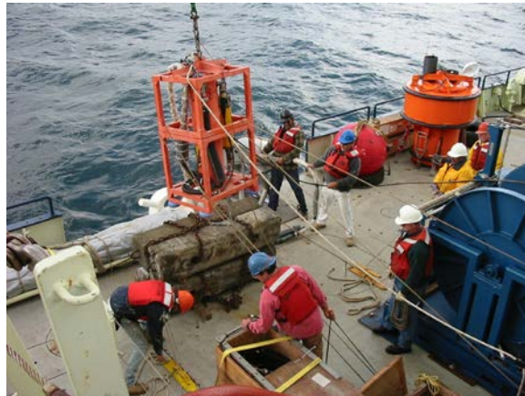
Deployment of the NRL Acoustics Division's bottomed vertical line array receiver and digital acquisition unit during the T-MAST 02 Field Test near the west coast of Scotland in July 2002. (Courtesy Dr. Michael Nicholas)
