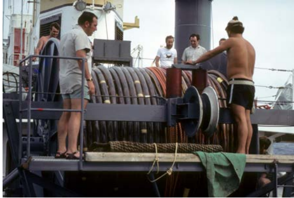
Preparation for deployment of towed horizontal line array of receiving hydrophones from HMNZS Tui during NRL testing in 1979 (Courtesy Dr. B.B. Adams)
