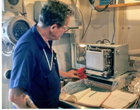
Jason Husty Taylor adjusting paper chart recorder for the monitoring hydrophone during NRL testing aboard HMNZS Tui in 1979 (Courtesy Dr. B.B. Adams)
