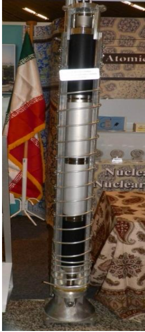
Figure 6: A photo of a model of the IR-1 centrifuge in Iran, showing four aluminum rotor tubes and three bellows. The top and bottom tubes are painted black, possibly intended to help control the temperatures along the rotor assembly. The small tubing wrapped around the outside of the centrifuge is for water flow related to controlling the temperature along the rotor assembly. The IR-1 centrifuge is the same as Pakistan’s P-1 centrifuge. Iran obtained this centrifuge design from the A.Q. Khan network.
