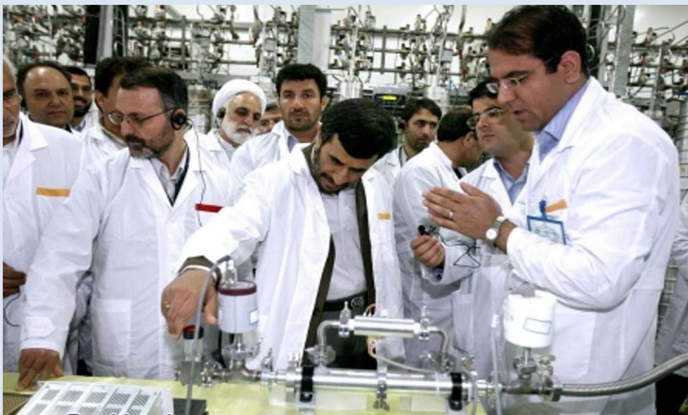
Figure 14: President Ahmadinejad examines gas centrifuge equipment, which includes an older MKS pressure transducer (next to his right hand) during a visit to the Natanz pilot fuel enrichment plant in 2008. In the background is an IR-1 gas centrifuge cascade which contains many more recent (mid-2000s) models of MKS pressure transducers. The MKS pressure transducers are controlled on dual-use lists; the white pressure transducer on the right in the foreground was not on the dual use list at the time it was sold to Iran.
