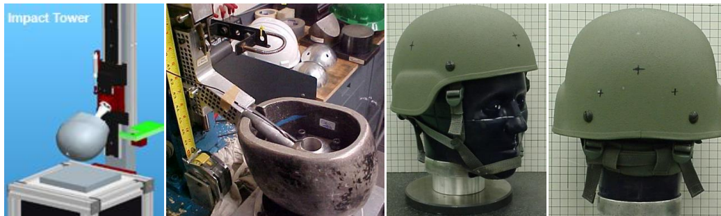
Figure 1. Monorail drop tower (left), DOT headform (center left), and ACH blunt impact locations (+) on a NOCSAE headform (center right and right)
