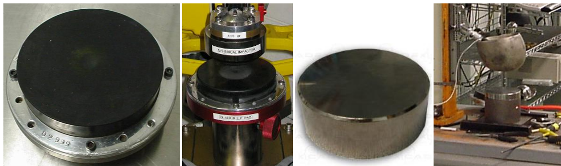
Figure 5. MEP monorail drop test setup with a hemispherical impactor (left and center left). Flat anvil monorail drop test setup with a DOT headform (right and center right).
